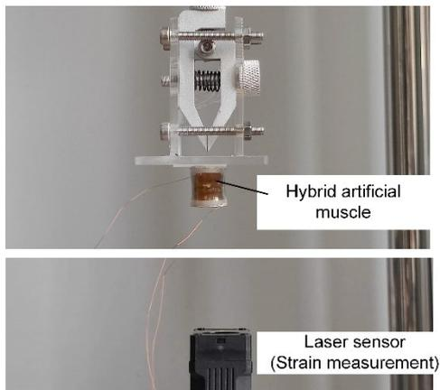
**Fig. S2. Experimental setup for strain measurement.**
