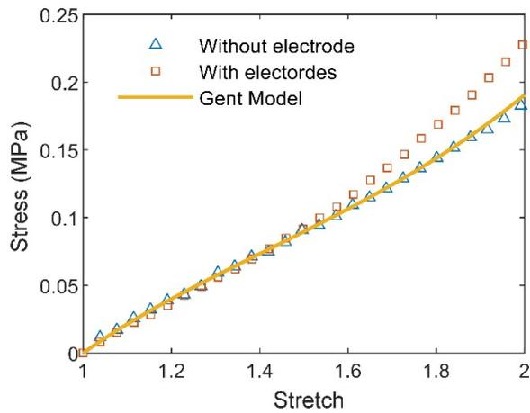
**Fig. S7.** Uniaxial tensile test curves of DEA with electrodes and DEA without electrodes, and the result of Gent model.
