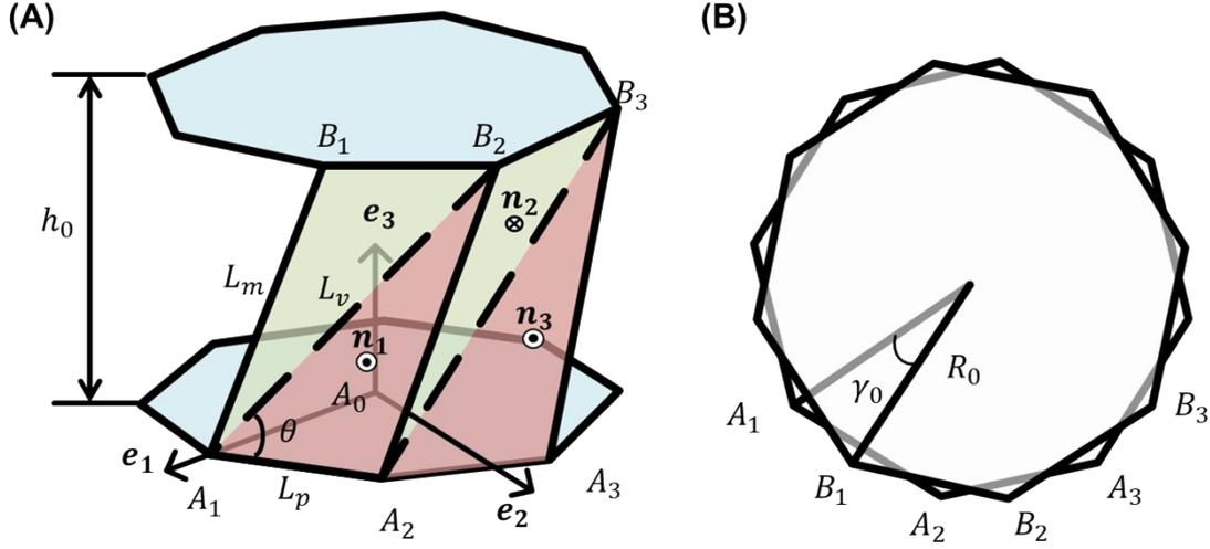
**Fig. S4.** Geometry of a Kresling origami unit at initial state. (A) 3D view. (B) Top view.
