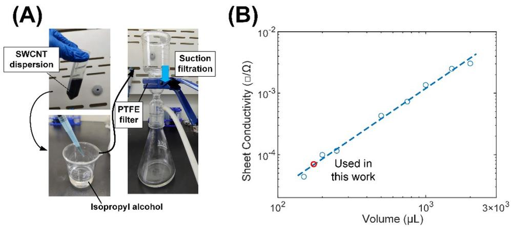
**Fig. S1. Fabrication and performance characterization of SWCNT electrode.** (A) Fabrication processes of SWCNT electrodes. (B) Sheet conductivity as a function of the volume of the SWCNT dispersion used.
