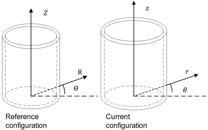
**Fig. S6.** Schematic figure for the reference and current configurations of a rolled DEA.
