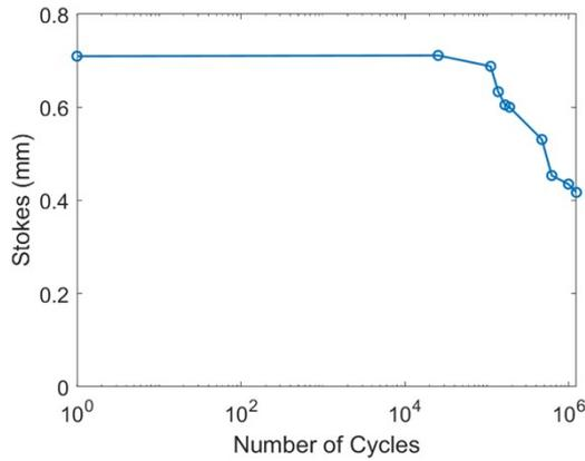
Fig. S8 Stroke of OHAM-QZ5 during cycling test at 1200 V and 125 Hz which is the resonance frequency of a new specimen.
