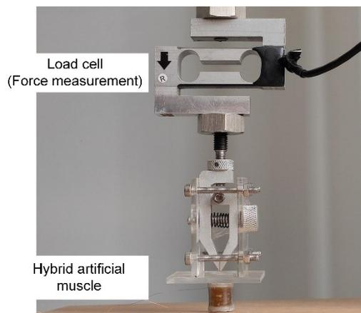
**Fig. S3. Experimental setup for and blocked force measurement.**
