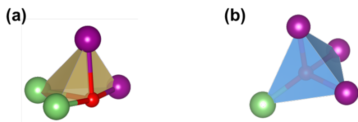
Fig. S2 Two four-coordinated oxygen configurations. (a) Oxygen is located at the edge of the tetrahedron (Oct-4); (b) Oxygen is located at the center of the tetrahedron (Tet-4).
