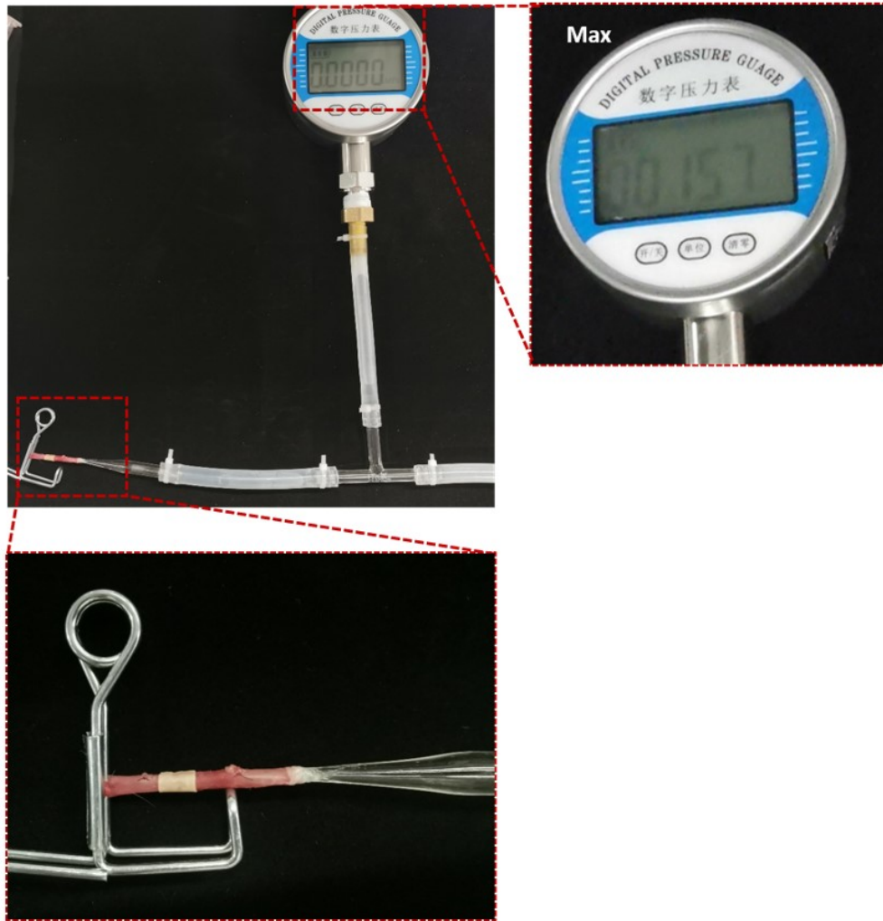
Figure S11. Bearing pressure of healed PCLUse tube on an aortaventralis. Performance of the self-manufacture manometry set to measure the bearing pressure of the leaking site in aortaventralis of rabbit and the maximum pressure as shown in the red dot rectangle.
