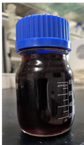
Fig. S2. Scale-up preparation of ANF from the macroscopical Kevlar aramid fibers.
