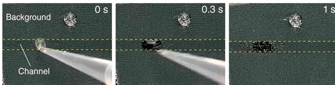
Figure S1: Time-lapsed images of water droplet wetting the silica particle-patterned channels on the PDMS-coated superhydrophobic fabric.
