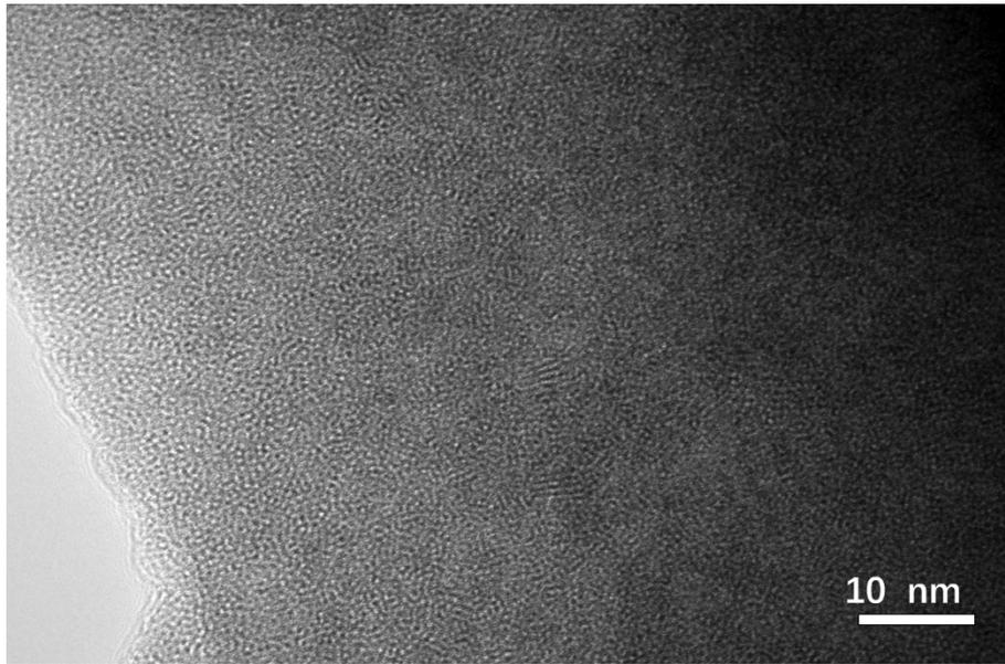
**Fig. S4** High resolution TEM image of pure MoS<sub>2</sub> film with amorphous nano-structure.
