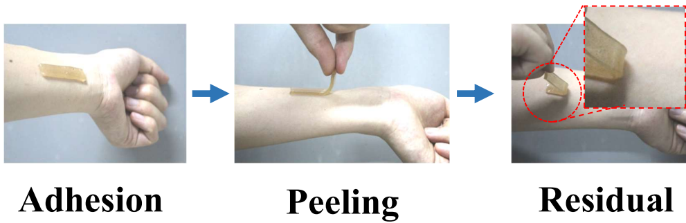
Fig. S11. Photographs of CS/PVA-PA-10BA hydrogel before and after adhering to the skin.
