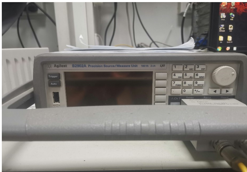
Figure S16. Physical photography of an Agilent Keysight B2900A Quick IV measurement system.
