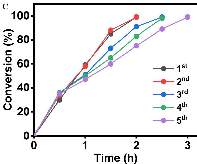
**Figure S8. Recycling processes of the catalyst and EG.** (A) Successive separation of the catalyst and EG after each cycle. (B) Conjugative addition of PET and EG after completion of each step. (C) Assessment of catalyst stability with PET deconstruction by using TBD:TFA (1:1). Reaction conditions: PET (1 eq.), catalyst (0.05 eq.), EG (10 eq.), 180 °C at 0-3 h.
