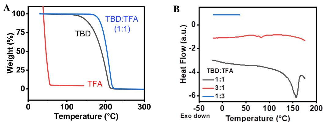
**Figure S18.** (A) Thermogravimetric analysis for TBD, TFA and TBD:TFA (1 : 1). (B) Dynamic Scattering Calorimetry (DSC) of different ratios (1:1, 3:1 & 1:3) of TBD:TFA.
