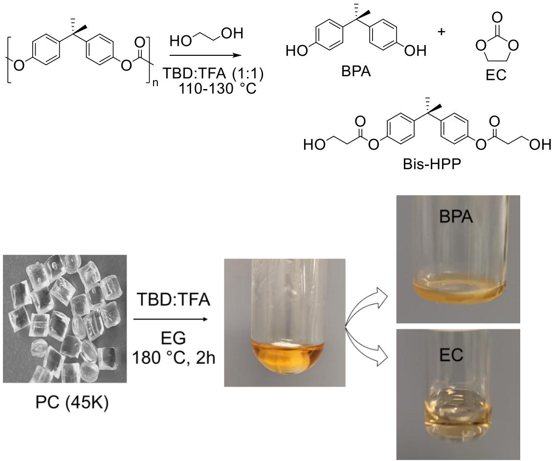
**Figure S6. Deconstruction process of PC.** PC (1eq.) pellets were completely deconstructed by using TBD:TFA (0.05 eq.) at 130 °C for 2 h.
