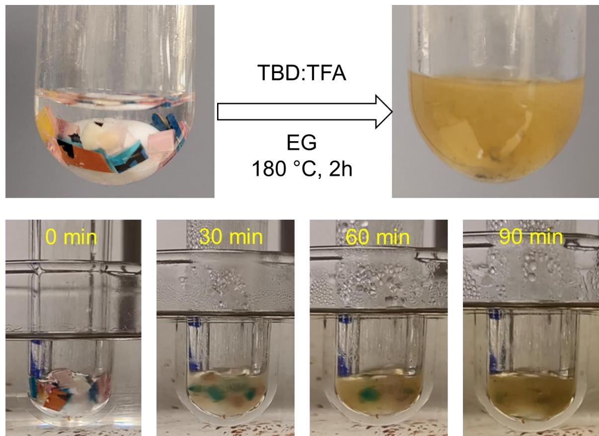
**Figure S12.** Deconstruction of colored PET bottle at different time intervals using TBD:TFA as a catalyst and EG as a substrate. At a certain interval, the colored fragment disappears, and the formation of a solution indicates the progression of the PET bottle deconstruction.
