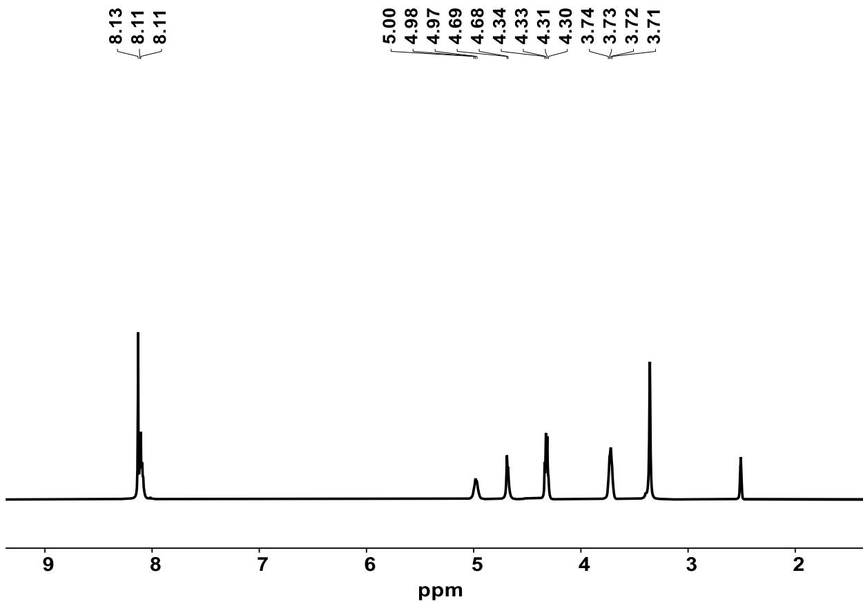
**Figure S68.** <sup>1</sup>H NMR spectrum of the mixture of BHET monomer and dimer from the deconstruction of carpet (0.5 g), EG (1.61 g), and TBD:TFA (0.035 g), as a catalyst at 180 °C (DMSO-d<sub>6</sub>, 400 MHz, 298 K).
