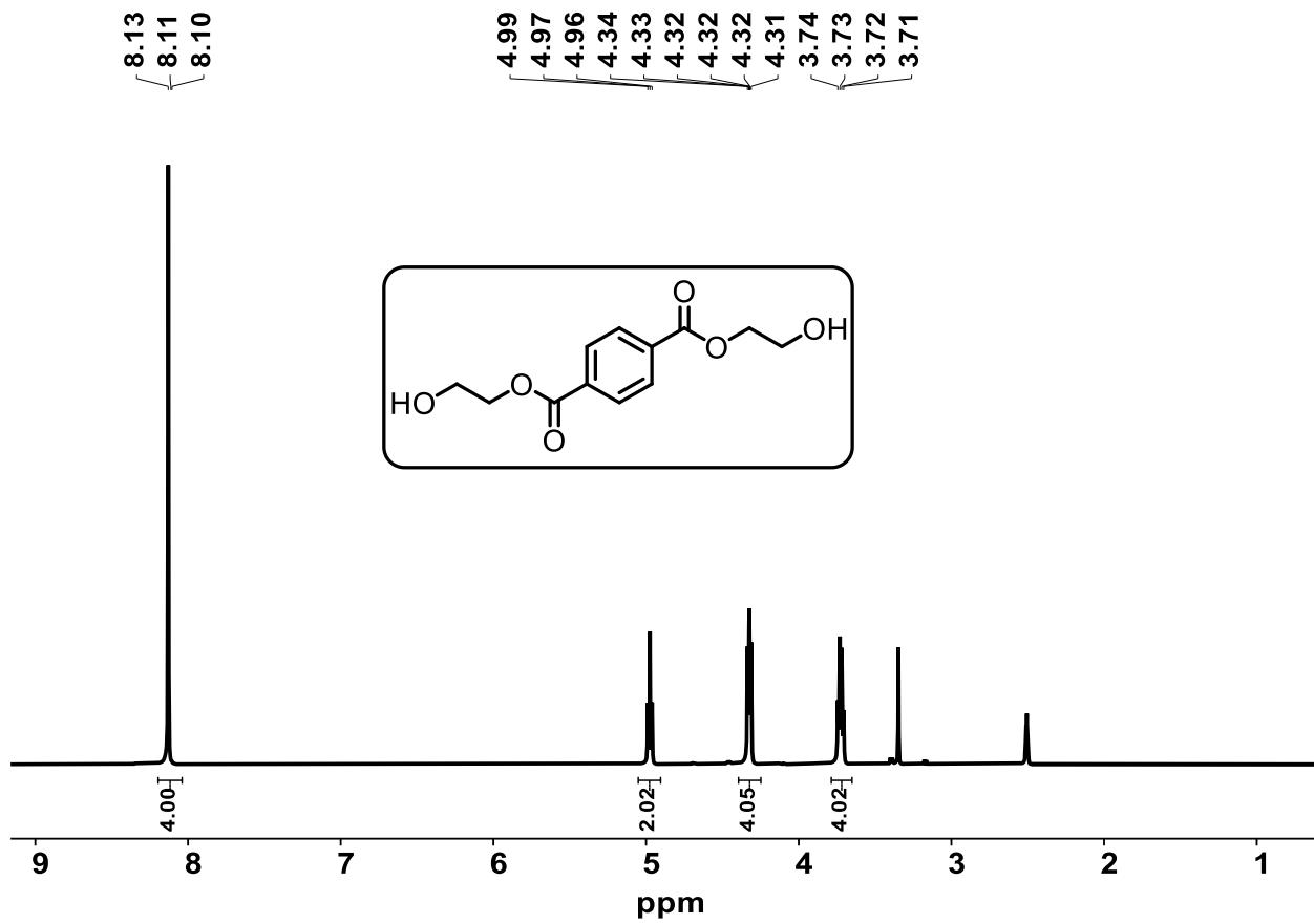
**Figure S26.**  $^1\text{H}$  NMR spectra of the BHET ( $\text{DMSO-d}_6$ , 400 MHz, 298 K).
