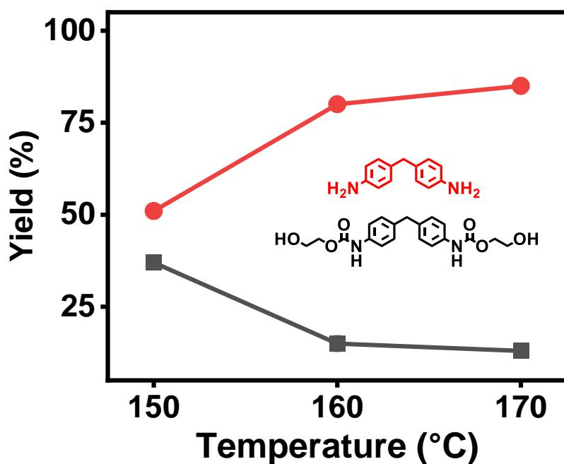
**Figure S7.** Effect of temperature on PU deconstruction. At low temperature (150 °C), MDA and BMDC yields equally but at 170 °C more MDA (80%) yields than BMDC (17%).
