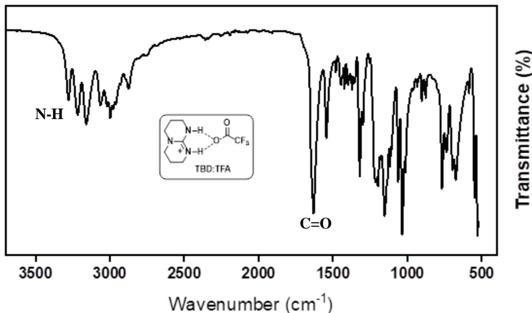
**Figure S15.** FTIR spectrum of TBD:TFA (1:1). In the IR spectrum, the presence of ketone ( $\text{C=O}$ ) and various N-H peaks as well as the disappearance of the acid peak indicate the successful formation of the TBD:TFA
