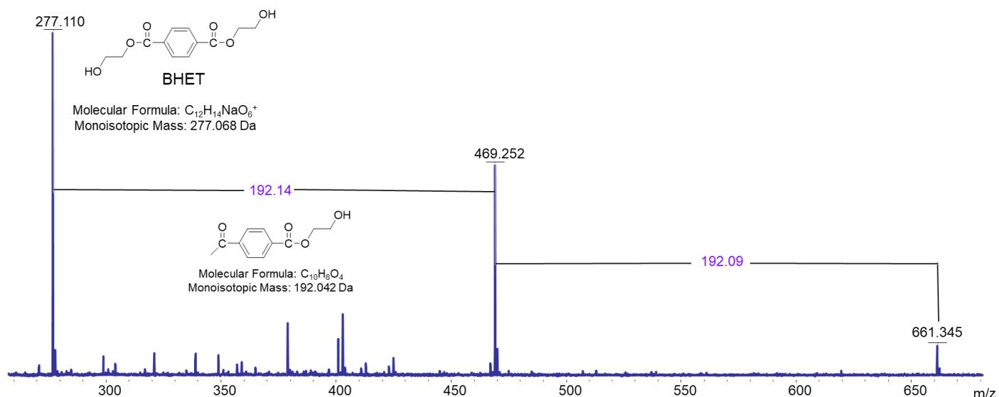
**Figure S28.** MALDI-TOF of the crude products from the deconstruction of PET. The peak indicates the formation of BHET with high yield, and some mixture of monomer and dimer also formed.
