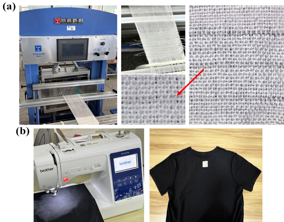
Figure S13. The processing and structure of textile. (a) Fiber working electrodes and reference electrodes as weft yarns for this work, polyester threads as weft yarns for the other parts of the filling and warp parts. (b) The process and diagram of sewing fabric into clothes
