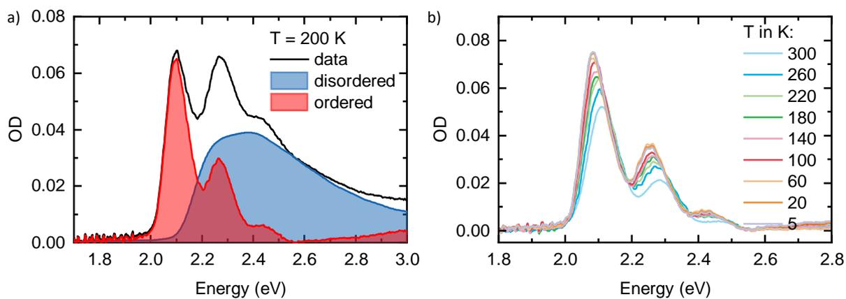
**Figure S3:** (a) example of the spectral decomposition of the absorption at 200 K (black line) into absorption from non-aggregated chains (blue area) and from aggregated chains (red area). The spectrum of the non-aggregated chains is obtained from temperature-dependent absorption measurements of PDOPT in a THF solution. (b) extracted absorption spectra of the aggregated chains.
