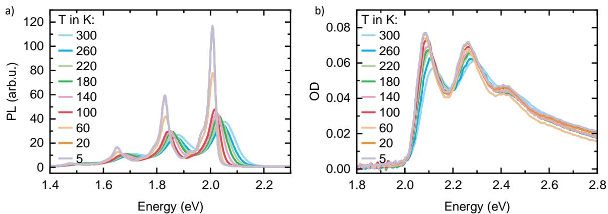
**Figure S1:** Temperature-dependent measurements of (a) PL and (b) Optical Density of the PDOPT thin film.
