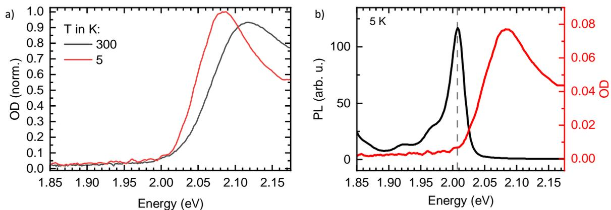
**Figure S2:** (a) Magnified range of the absorption onset at 300 K and 5 K. (b) PL and absorption at 5 K plotted on the same energy axis. The dashed line indicates the energetic position of the 0-0 PL peak extracted from the FC-analysis.
