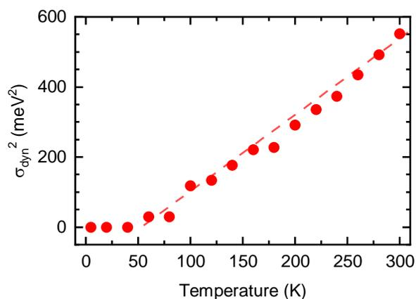
**Figure S5:** Contribution of the dynamic disorder (squared) to the line width of the absorption spectra as a function of temperature.
