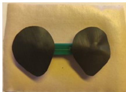
Figure S21. The pictures of electrodes on the wireless module (BMD101, NeuroSky) for electrocardiogram (ECG) and electromyogram (EMG) monitoring.
