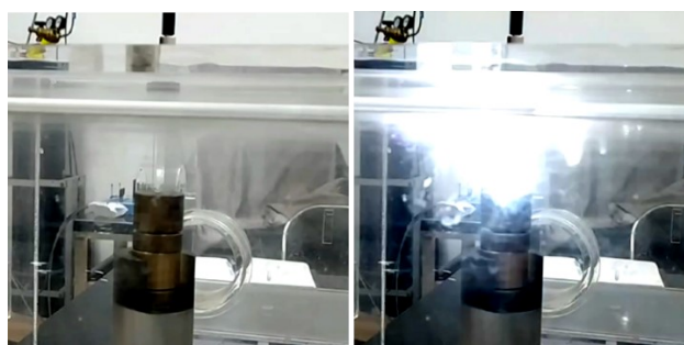
Figure S6. The detonation of BLG-1 with a laser irradiation ( P=13\text{W} , t=1\text{ms} , E=13\text{mJ} ).
