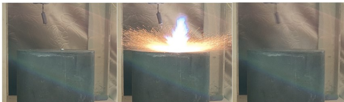
Figure S7. The detonation of 10 mg of BLG-1 in an aluminum crucible.
