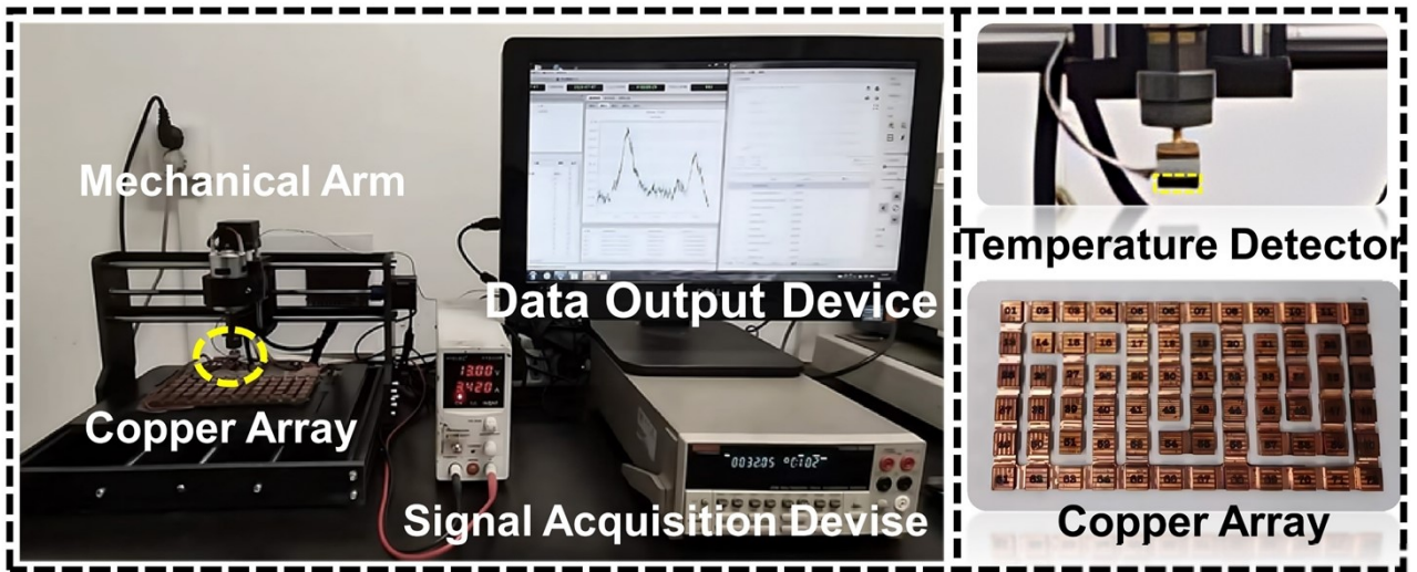
Fig. S18. The optical images of the dynamic thermal sensing temperature detection equipment.
