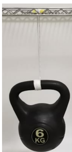
Figure S32. The photo of poly[TA-Ch] long-term weight-loading tests.
