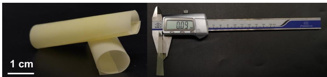
Figure S23. Poly[TA-Ce] film. (the thickness of film is 0.09 mm; TA/Ce = 10/1)
