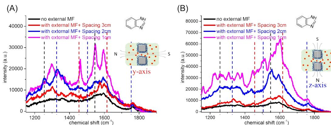
**Figure S4 Raman spectra of vertical dimer nanojunctions composite with benzimidazole under different strengths of the external magnetic force.** The strength of the magnetic force applied on the composite can be tuned by changing the spacing between the composite and the magnetic source (magnetic bar). Raman spectra of nanocomposites with two different morphologies of dimer nanojunctions, vertical and horizontal dimer nanojunctions, are shown in (A) and (B), respectively.
