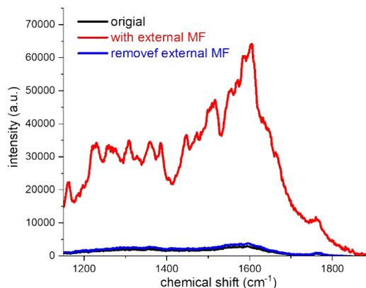
**Figure S19 The reproducibility test of nanocomposites with magnetic materials for magnetic sensing application.** Through the change of Raman scattering spectrum changes with the change of external MF, it can be observed that after the external MF is removed, the rearrange of molecules around the dimer nanojunction returns to the original state. This allows these nanocomposites to be reused.
