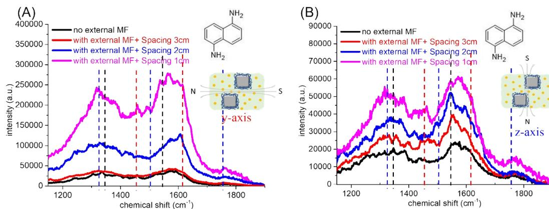
**Figure S3 Raman spectra of horizontal dimer nanojunctions composite with naphthalenediamine under different strengths of the external magnetic force.** The strength of the magnetic force applied on the composite can be tuned by changing the spacing between the composite and the magnetic source (magnetic bar). Raman spectra of nanocomposites with two different morphologies of dimer nanojunctions, vertical and horizontal dimer nanojunctions, are shown in (A) and (B), respectively.
