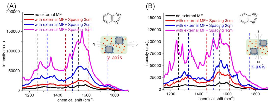
**Figure S5 Raman spectra of horizontal dimer nanojunctions composite with benzimidazole under different strengths of the external magnetic force.** The strength of the magnetic force applied on the composite can be tuned by changing the spacing between the composite and the magnetic source (magnetic bar). Raman spectra of nanocomposites with two different morphologies of dimer nanojunctions, vertical and horizontal dimer nanojunctions, are shown in (A) and (B), respectively.
