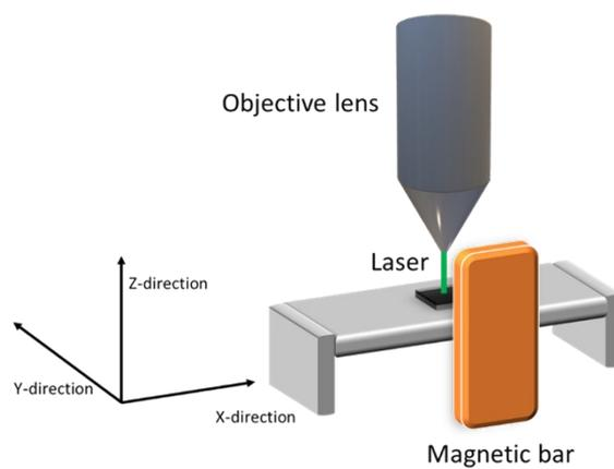
**Figure S1 Experimental setup for measurement the Raman spectra of dimer nanojunctions composite under different directions of the external magnetic force. (A) y-axis magnetic field: magnetic field parallel to the substrate; (B) z-axis magnetic field: magnetic field perpendicular to the substrate.**
