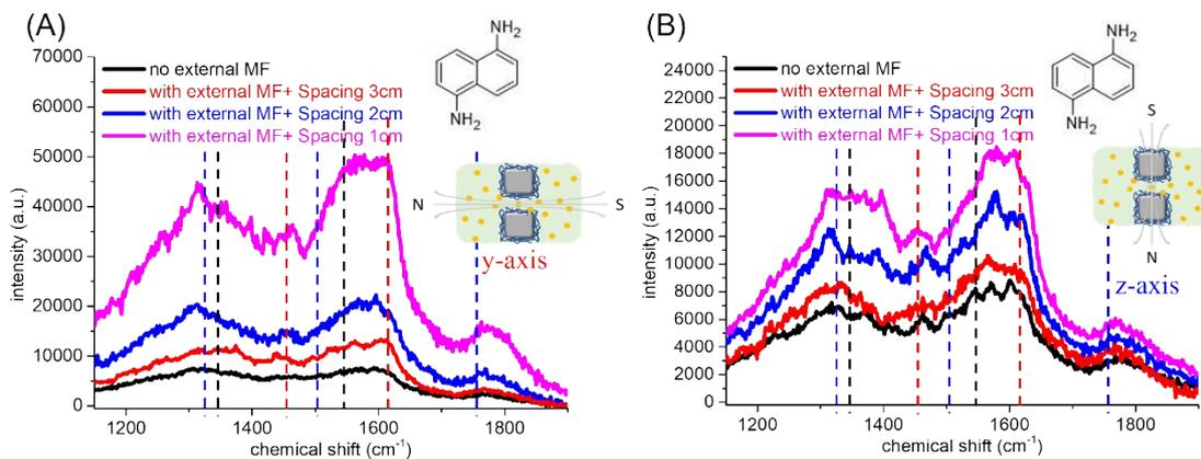
**Figure S2 Raman spectra of vertical dimer nanojunctions composite with naphthalenediamine under different strengths of the external magnetic force.** The strength of the magnetic force applied on the composite can be tuned by changing the spacing between the composite and the magnetic source (magnetic bar). Raman spectra of nanocomposites with two different morphologies of dimer nanojunctions, vertical and horizontal dimer nanojunctions, are shown in (A) and (B), respectively. □
