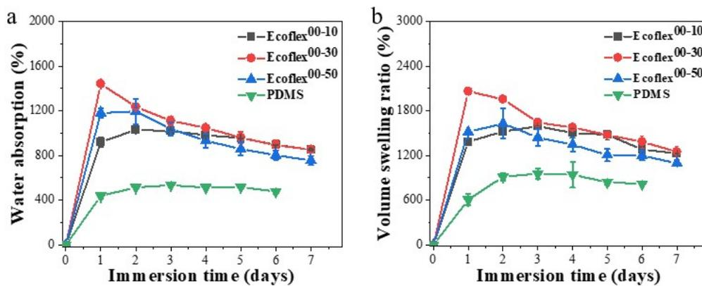
**Figure S2.** Swelling responses of Ecoflex<sup>00-10</sup>/NaCl composites using different water-unswellable polymers as the matrix. (a) Water absorption and (b) volume swelling ratio of different polymer composites with 50 wt.% NaCl in 300 mL of DI water under 60 °C. The base-to-cure agent ratio of PDMS is 30:1.
