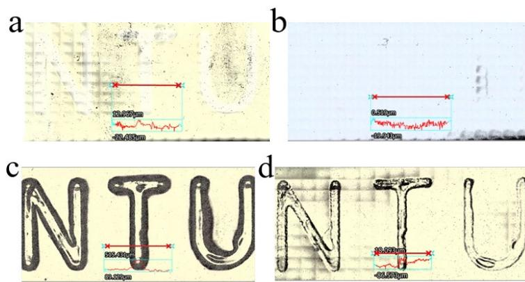
**Figure S15.** Optical images of the PDMS samples embedded with Ecoflex<sup>00-10</sup>/NaCl polymer composite after different treatments. (a) Braille “NTU” with a visual difference before soaking. (b) Braille “NTU” without a visual and tactile difference before soaking. (c) Braille “NTU” with a clear visual and tactile regulation after soaking. (d) Decrease of a visual and tactile regulation after drying.
