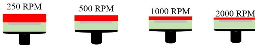
**Figure S12.** Schematic illustration of the control over the thickness of the liquid PDMS layer on top of PDMS samples with semi-embedded Ecoflex<sup>00-10</sup>/NaCl polymer composite by adopting different spin-coating speeds.
