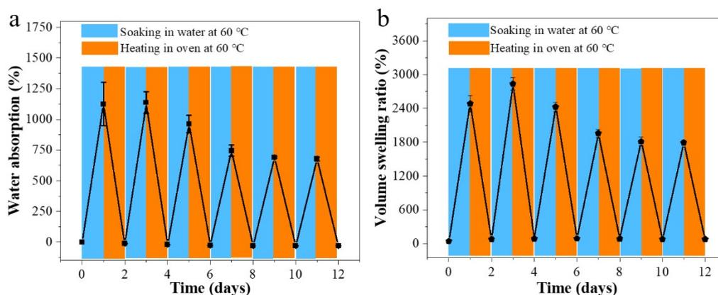
**Figure S7.** Characterization of the swelling repeatability of Ecoflex<sup>00-10</sup>/NaCl polymer composite with 50 wt.% NaCl under cyclic soaking-drying conditions. (a) Water absorption and (b) volume swelling ratio during multiple immersion and drying cycles.
