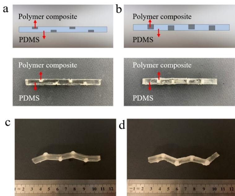
**Figure S10.** Swelling-induced zigzag-shaped bending of PDMS strips. (a-b) Schematic illustration and the physical models of the PDMS strips with semi-embedded Ecoflex<sup>00-10</sup>/NaCl polymer composite strips of different thicknesses. (c-d) The fully swelled configurations of the samples in (a) and (b), respectively.
