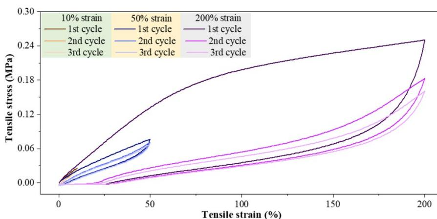
**Figure S6.** Stress-strain curves of the Ecoflex<sup>00-10</sup>/NaCl polymer composite with 50 wt.% NaCl during the first three loading-unloading cycles under maximum 10%, 50% and 200% tensile strains.
