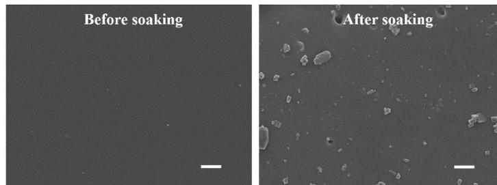
**Figure S8.** Representative SEM images of the Ecoflex<sup>00-10</sup>/NaCl polymer composite surface morphologies before and after soaking in DI water. The swelled sample was dried in oven before imaging. Scale bars: 10  $\mu\text{m}$ .
