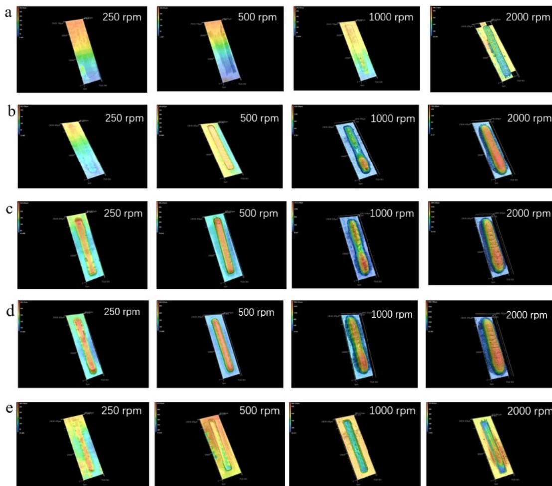
**Figure S13.** Surface morphologies of the sample that covered with PDMS of different thicknesses under different swelling states. (a) Before soaking in water. (b) After soaking in water for 1 day. (c) After soaking in water for 2 days. (d) After soaking in water for 3 days. (e) After drying.
