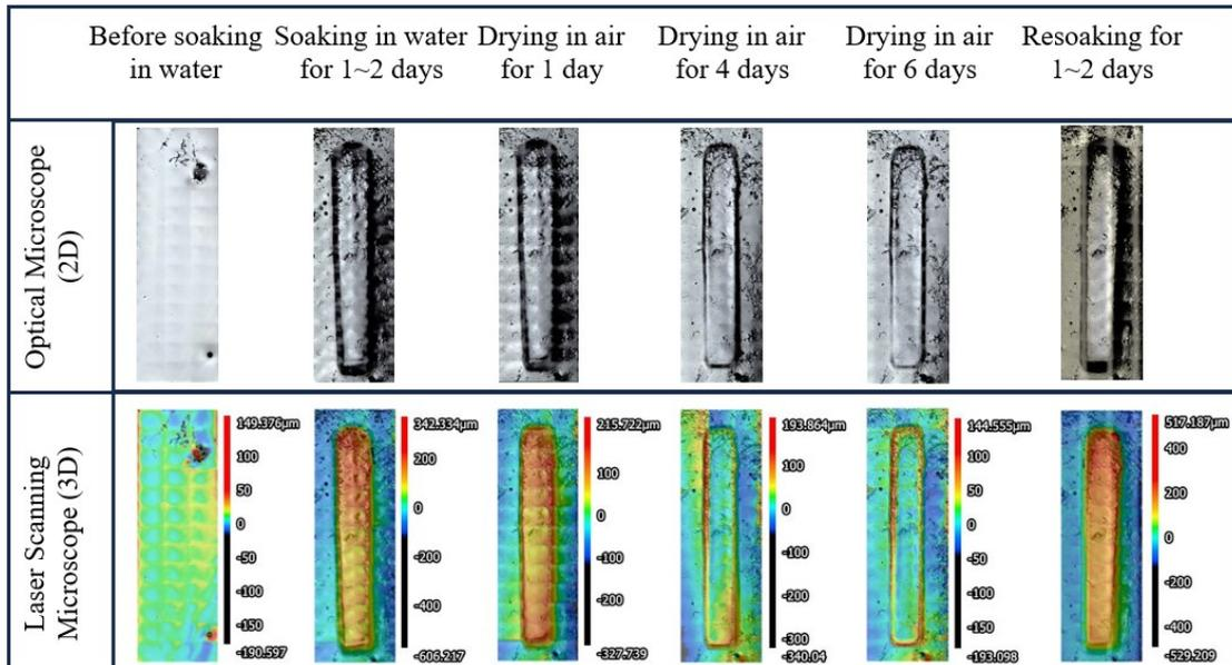
**Figure S11.** The optical microscopy and laser scanning microscopy images of Braille surface before and after soaking in water, drying in ambient air, and re-soaking in water.
