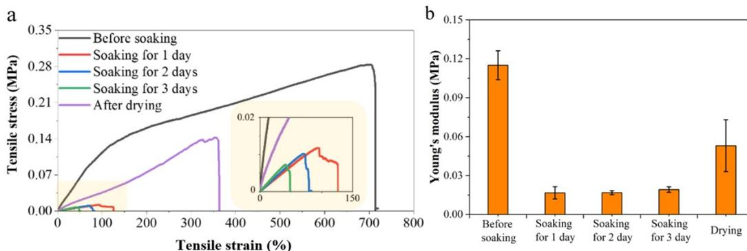
**Figure S5.** Characterization of the mechanical properties of the Ecoflex<sup>00-10</sup>/NaCl polymer composite. (a) Representative stress-strain curves of the sample at different swelling states. (b) Young's modulus of the sample after different treatments.
