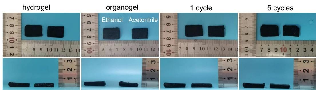
**Figure S10.** The volume evolution of PANI/SA gels during solvent displacement.
