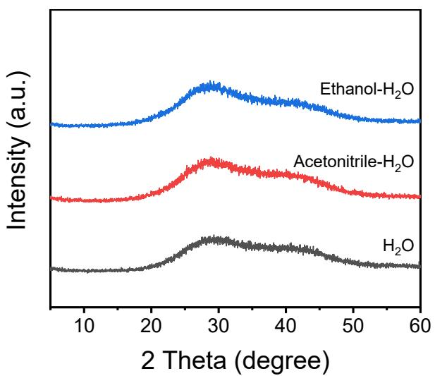
**Figure S11.** XRD patterns of the PANI/SA hydrogel after 5 solvent displacement cycles.
