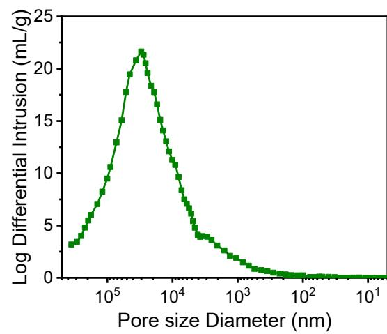
**Figure S2.** Pore diameter distribution of the PANI/SA aerogel.
