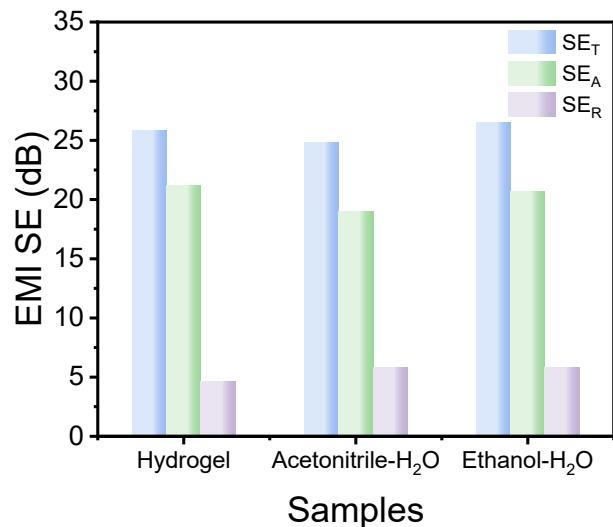
**Figure S13.** SE<sub>A</sub>, SE<sub>R</sub>, and SE<sub>T</sub> of the PANI/SA hydrogels after 5 solvent displacement cycles.
