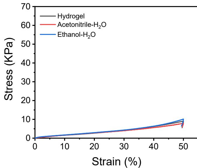
**Figure S12.** compression stress–strain curves of PANI/SA hydrogels after 5 solvent displacement cycles.
