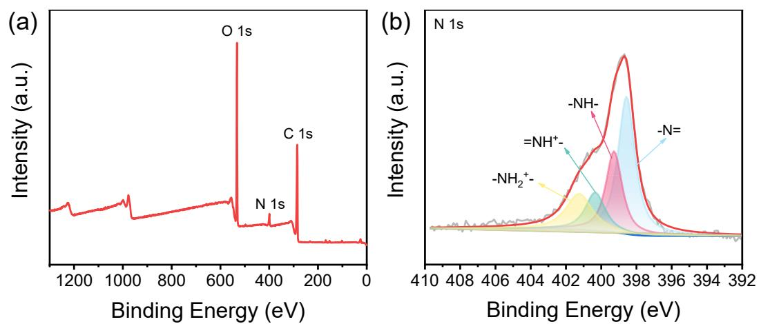
**Figure S3.** (a) XPS survey and (b) N 1s spectrum of PANI/SA aerogel.
