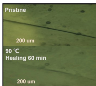
Fig. S14 Optical microscopy images of the scratched PU-5/5 film in healing process at 90 °C.
