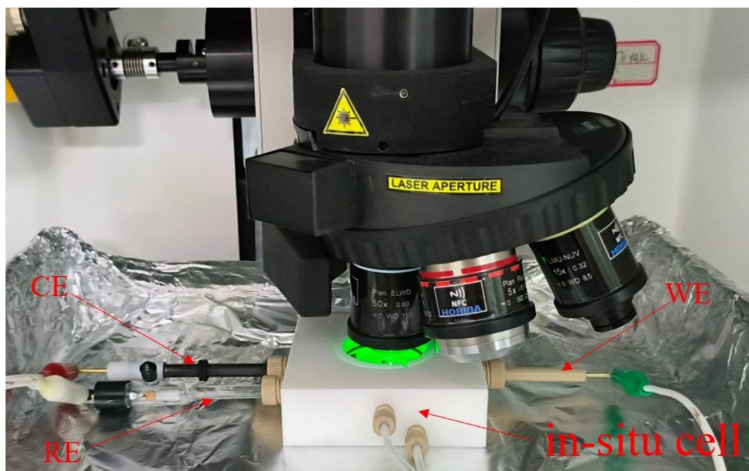
Fig. S21 Photograph of the in situ Raman testing setup. WE: working electrode, RE: reference electrode, and CE: counter electrode, respectively.
