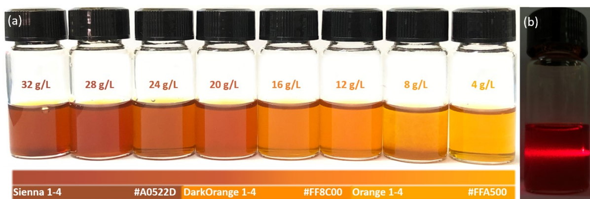
Supplementary Fig. 5: Photograph records of the NiFe-LDH NSs dispersed in formamide. (a) The 4–32 g/L concentrations of NiFe-LDH NSs and (b) the Tyndall effect of 28 g/L NiFe-LDH NSs colloidal suspension.
