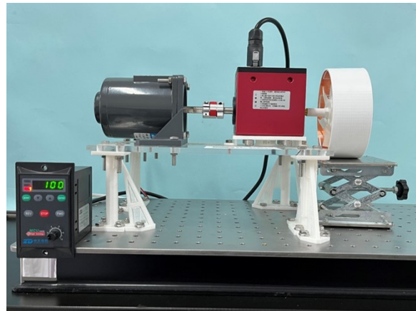
Figure S11. The test platform for torque measurement.
