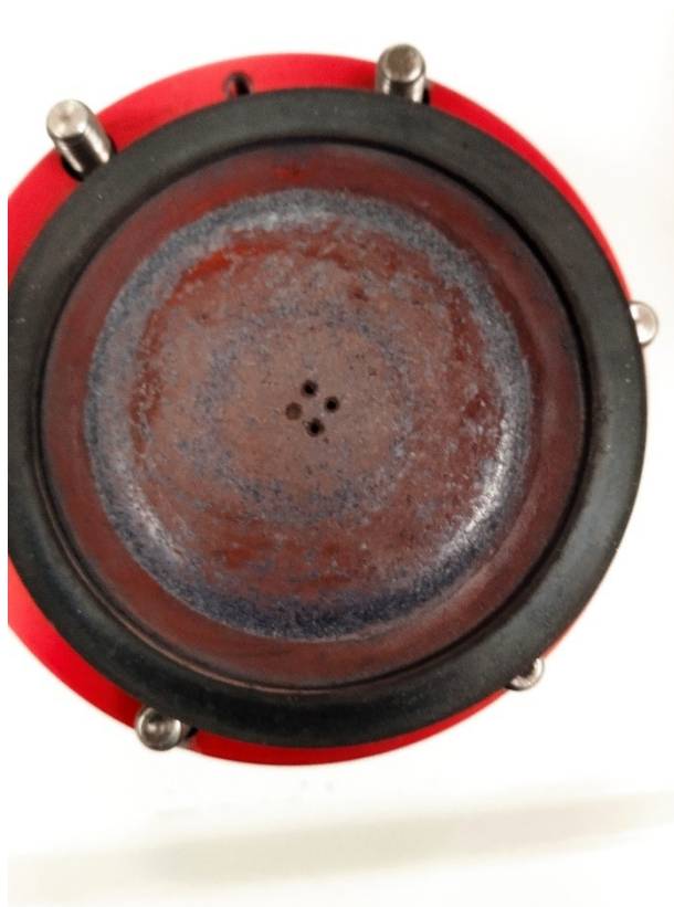
Fig. S4: Photograph of the lid after opening the milling chamber after the MSR reaction showing most probably red selenium powder
