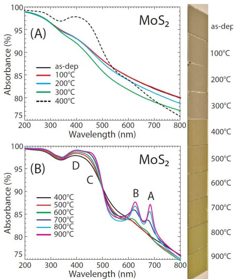
**Figure S1** Absorbance spectra of MoS<sub>2</sub> thin films deposited on transparent fused quartz substrates. The excitonic features A, B, C, and D are also indicated.
