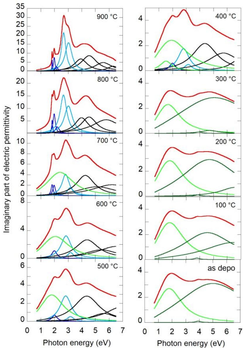
**Figure S2** Spectral deconvolution of MoS<sub>2</sub> electric permittivity along the amorphous to 2H MoS<sub>2</sub> crystalline transition. Presented are the imaginary parts and their particular contributions.
