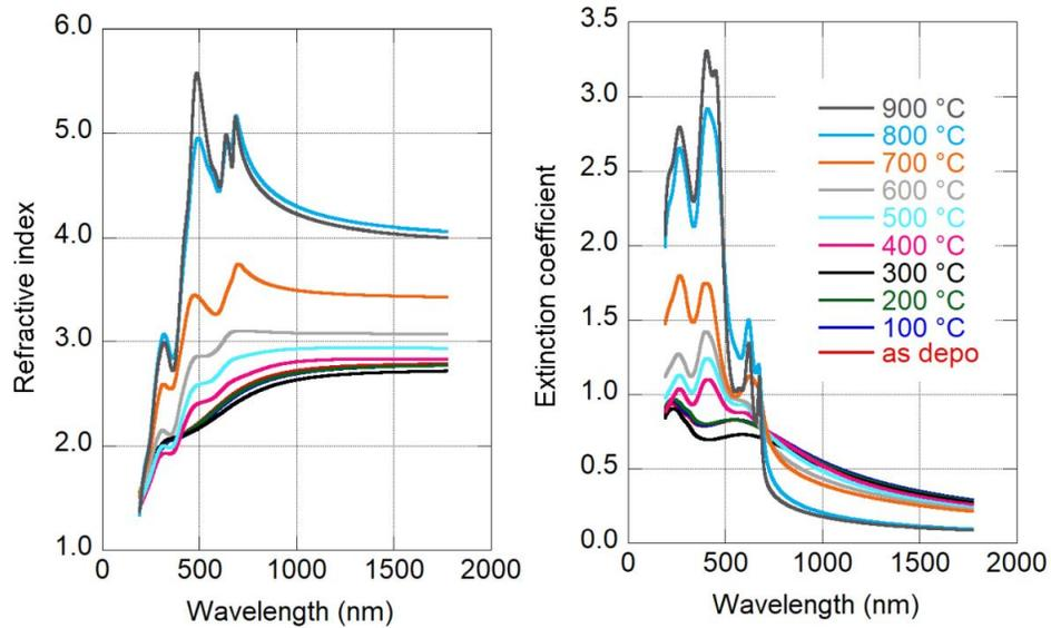
**Figure S3** Spectral dependence of refractive index and extinction coefficient of MoS<sub>2</sub> of as-deposited and annealed films.
