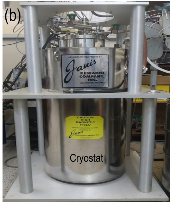
S9: Electrical measurement device. (a) Four-probe contact and (b) Cryostat
