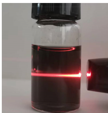
Figure S2. Dindar optical effect of V_4C_3 NSs dilute solution under laser pointer irradiation.
