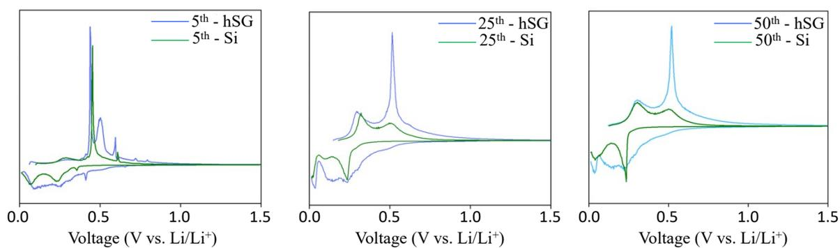
**Figure S8.** Comparison of dQ/dV curve of hSG and Si NWs at 5<sup>th</sup>, 25<sup>th</sup> and 50<sup>th</sup> cycle (at 0.2 C).
