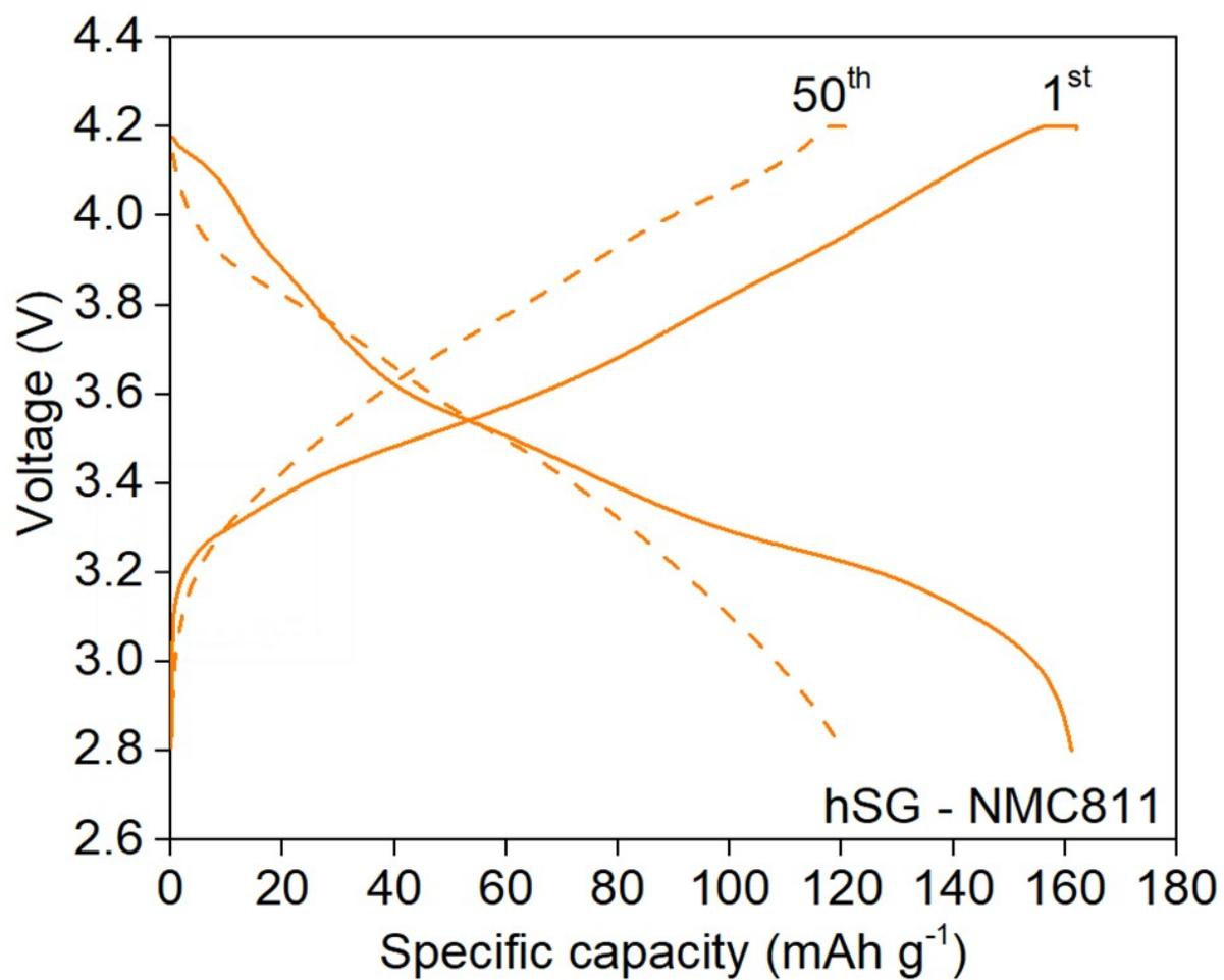
**Figure S10.** Voltage – specific capacity plot of hSG – NMC811 cell after 1<sup>st</sup> and 50<sup>th</sup> cycled at 0.2 C.
