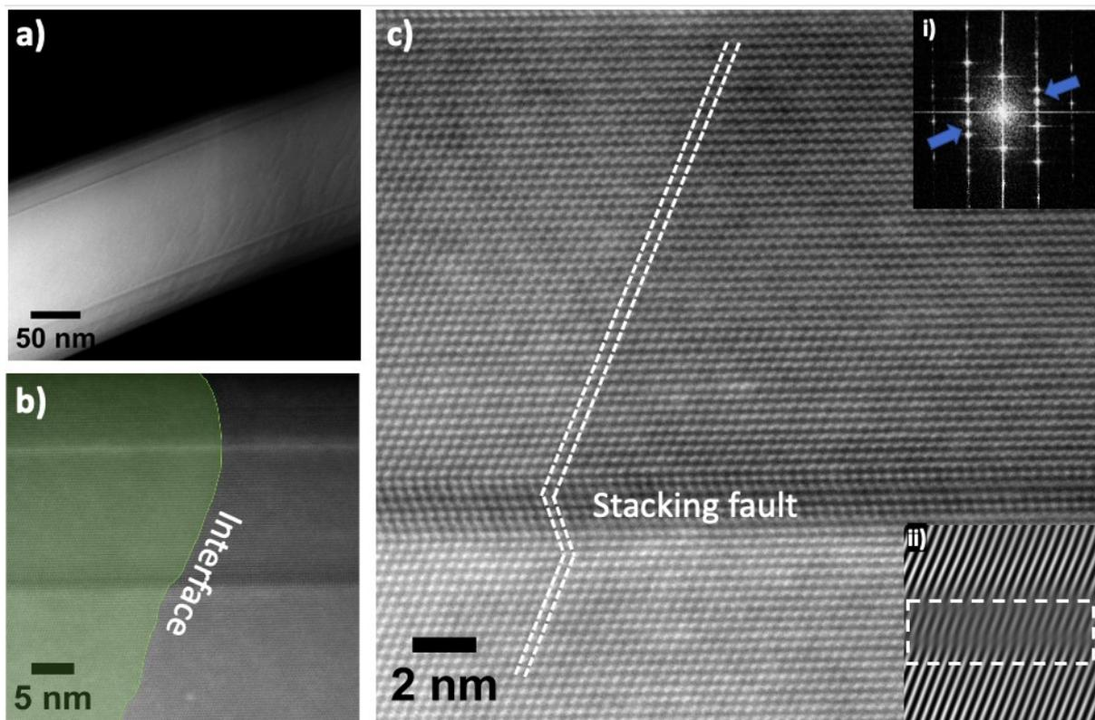
**Figure S3.** (a) HAADF-STEM image of hSG NW viewed from  $\langle 110 \rangle$  orientation. (b) High-resolution image, heterointerface highlighted by the green overlay, showing defect across the Si-Ge segment. (c) Atomic-resolution image of the heterointerface indicating SF marked by the white dashed lines. Insets are (i) FFT spots and (ii) IFFT image corresponding to the regions of SF.
