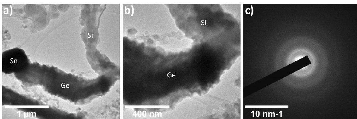
**Figure S7.** TEM analysis of the hSG anode at the 5<sup>th</sup> cycle (a) low magnification TEM image of the Sn, Si and Ge segments. (b) high magnification of Si and Ge segments. (c) Diffraction pattern of b with both segments now amorphous.
