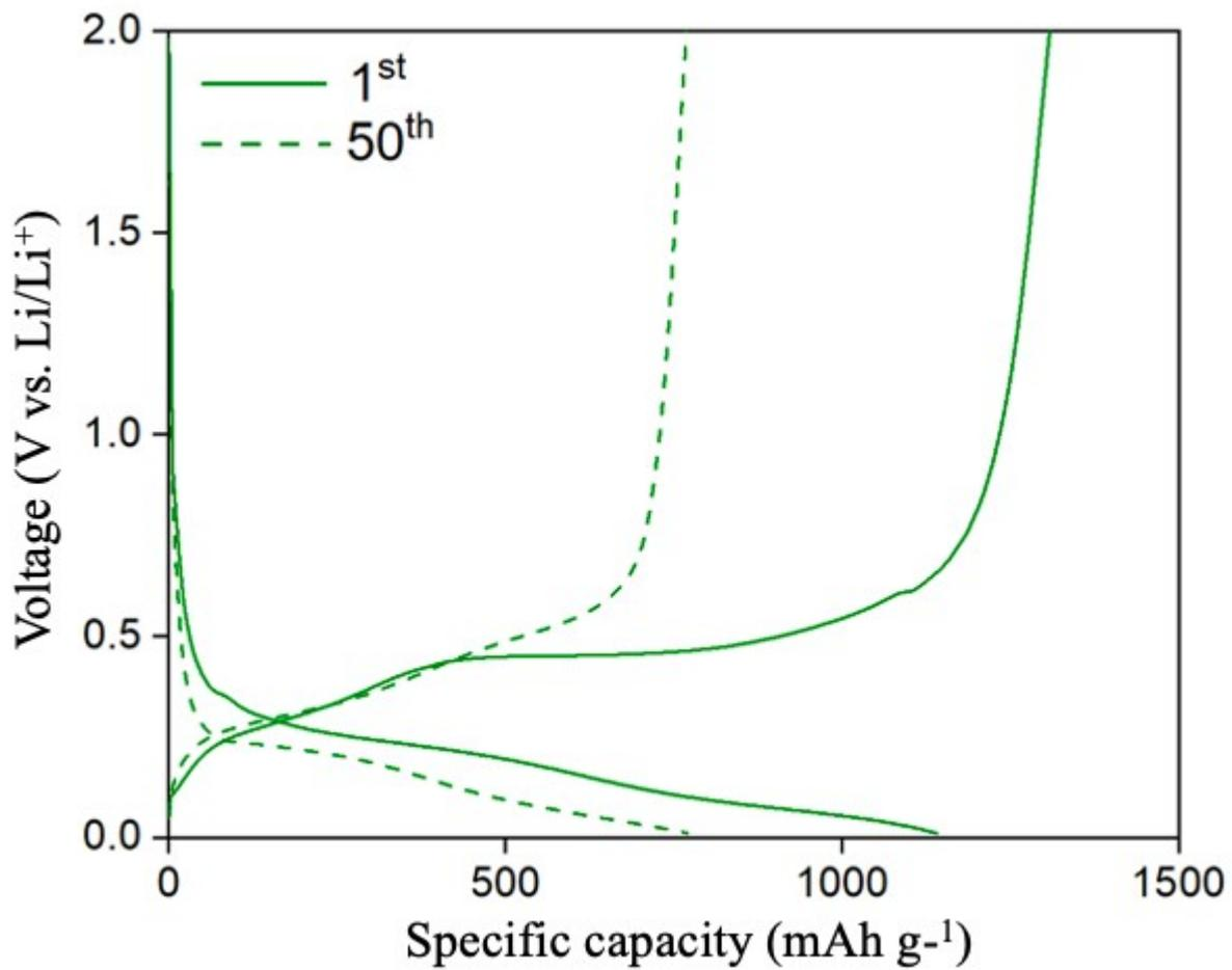
**Figure S4.** Voltage - Specific capacity profile of Si NWs (slurry) for 1<sup>st</sup> and 50<sup>th</sup> cycle at 0.2 C.
