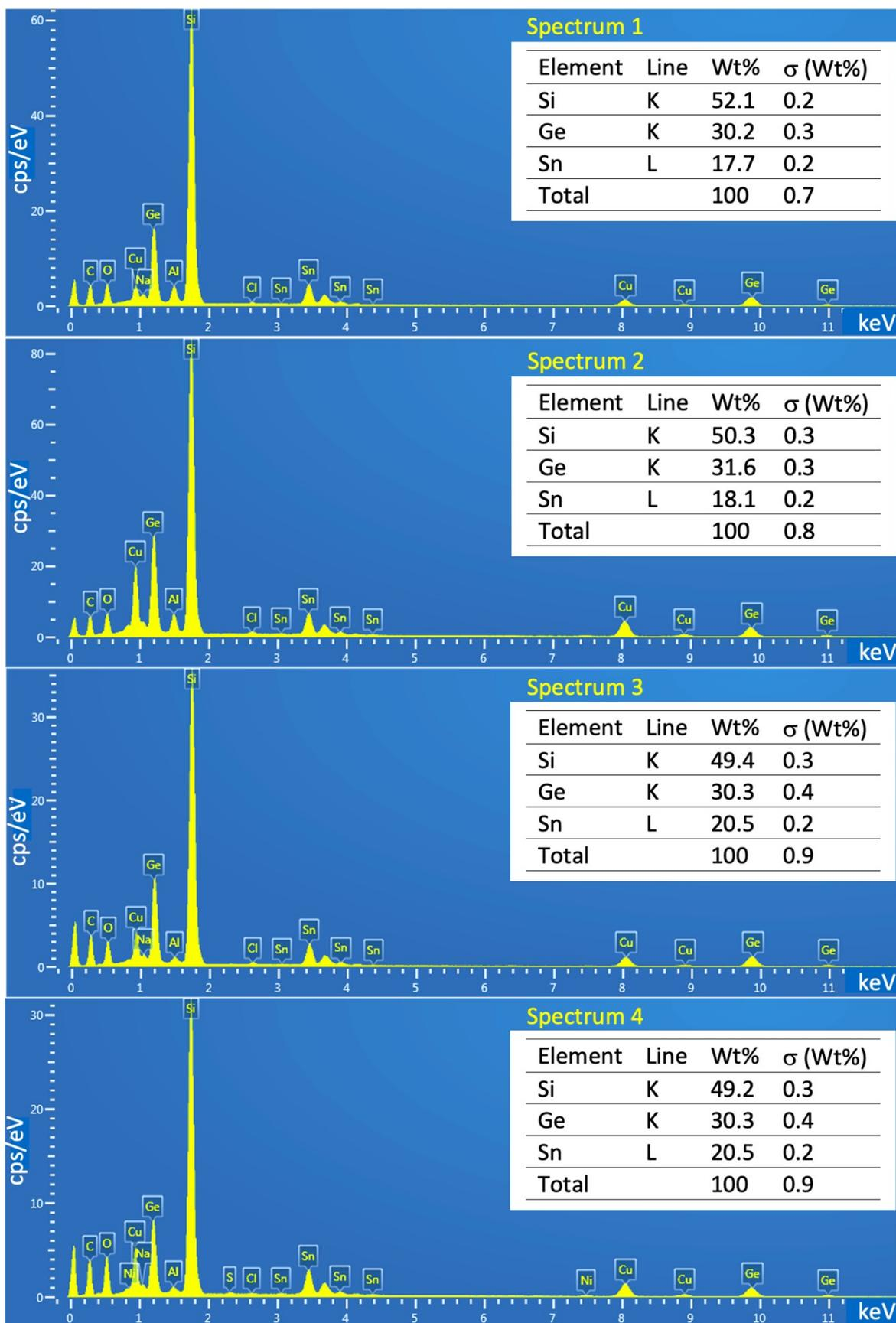
**Figure S1.** Quantitative EDX estimation of the % weight of Si, Ge and Sn from multiple areas of the anode. The mean value was obtained (Sn:Si:Ge weight % ratio is: 18:50:32).
