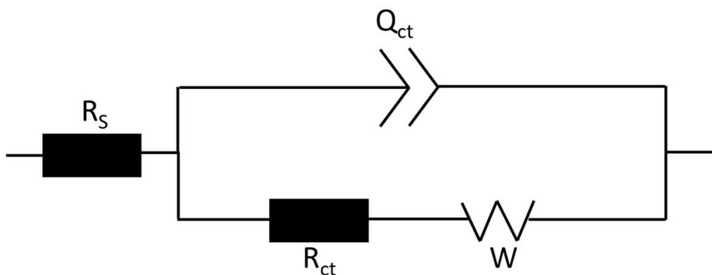
**Figure S5.** Fitting circuit used for EIS analysis.
