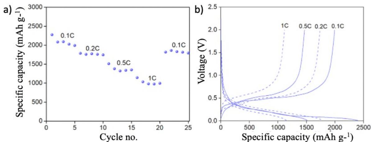
**Figure S6.** (a) Rate capability test and (b) corresponding voltage – specific capacity plot of hSG NWs at various C-rates.
