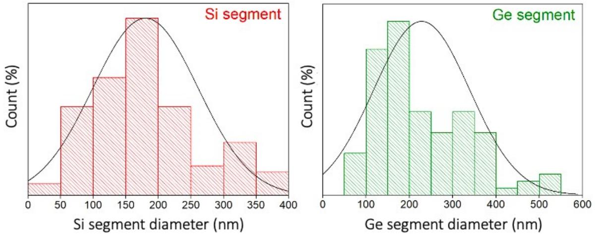
**Figure S2.** Histograms representing NW diameter distribution of Si and Ge segment in hSG NWs. Each distribution was obtained by direct counting method, measuring the diameters for 200 NWs from SEM images.
