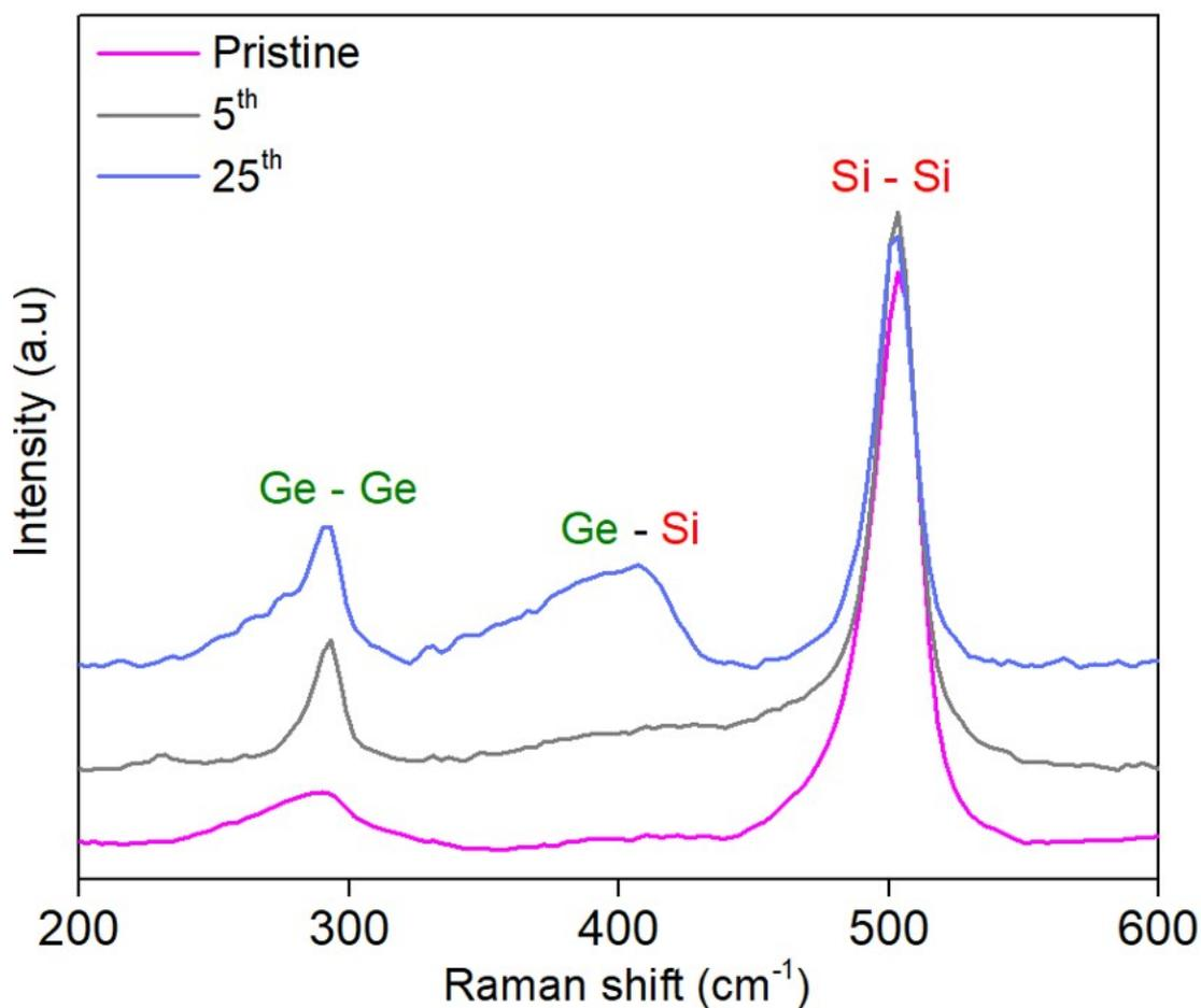
**Figure S9.** Raman spectroscopy analysis of hSG NWs before cycling (pristine), after 5<sup>th</sup> and 25<sup>th</sup> cycle.
