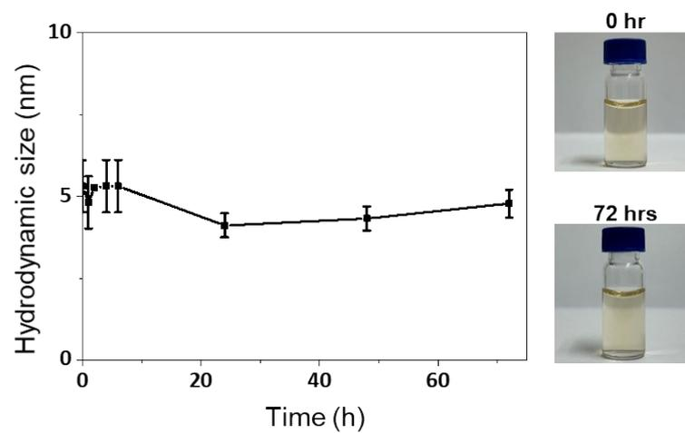
**Figure S8.** Colloidal stabilities of UMIOs measured in physiological saline.
