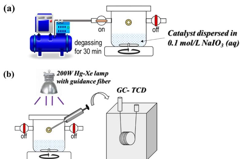
**Supplementary Fig. 7** Schematic diagram of the apparatus for the photo-oxidation of water in  $\text{NaIO}_3$  aqueous solution: (a) degassing, (c) UV irradiation, sampling, and quantification.
