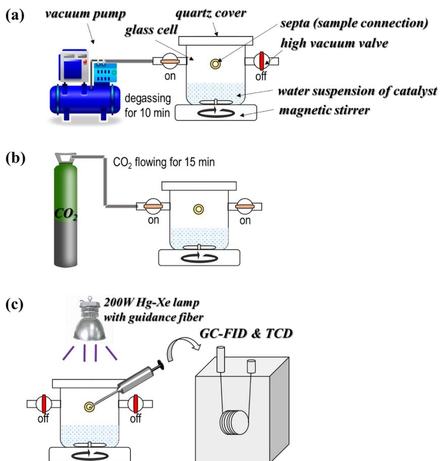
**Supplementary Fig. 6** Schematic diagram of the apparatus for the photo-reduction of CO<sub>2</sub>: (a) degassing, (b) CO<sub>2</sub> flowing, (c) UV irradiation, sampling, and quantification.
