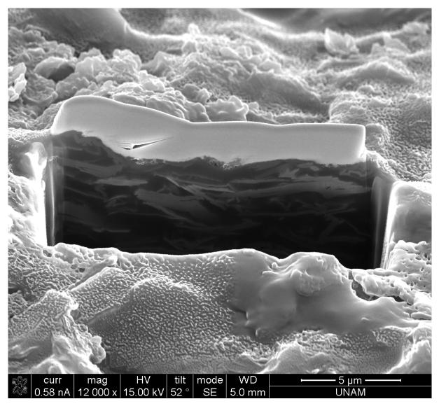
Figure S 29. SEM image of 10% APTES-rGO in coating.
