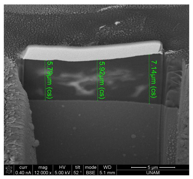
Figure S 25. SEM image of 5% APTES-rGO in coating.
