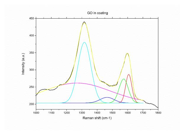
Figure S 7. Curve-fits to Raman spectra for rGO in coating. Gauss fits.
