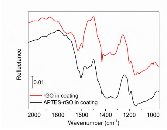
Figure S 4. FTIR spectra of coating containing APTES-rGO (black line) and not-containing APTES-rGO (red line).
