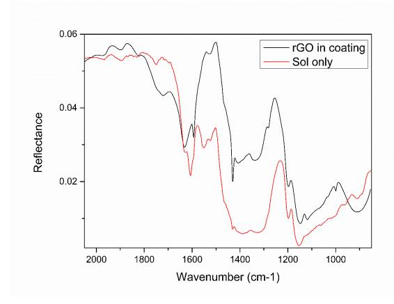
Figure S 5. FTIR spectra of coating containing rGO (black line) and not-containing APTES-rGO (red line).
