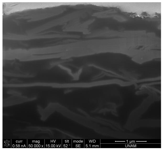
Figure S 30. SEM image of 10% APTES-rGO in coating.
