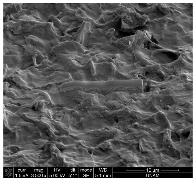
Figure S 34. SEM image of 5% rGO in coating.
