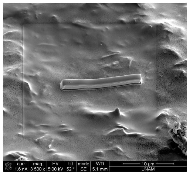
Figure S 22. SEM image of 5% APTES-rGO in coating.
