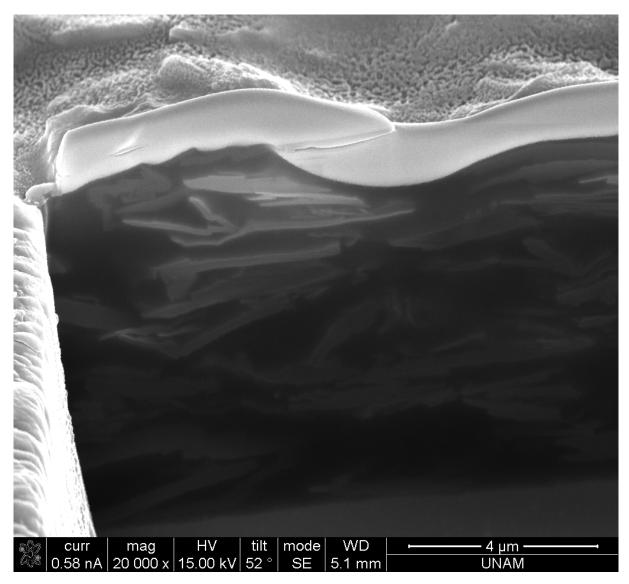
Figure S 33. SEM image of 10% APTES-rGO in coating.
