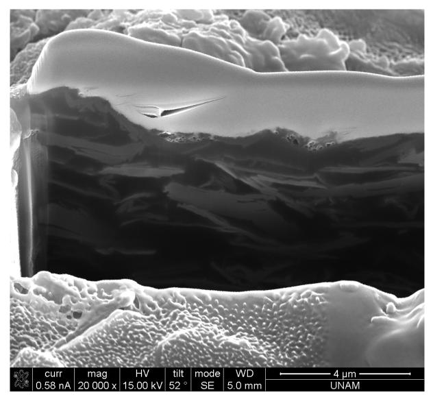
Figure S 28. SEM image of 10% APTES-rGO in coating.
