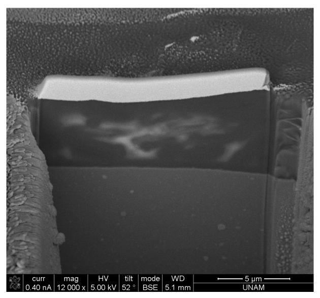
Figure S 24. SEM image of 5% APTES-rGO in coating.
