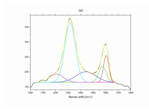
Figure S 6. Curve-fits to Raman spectra for GO. Gauss fits.
