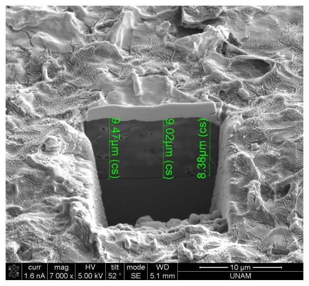
Figure S 37. SEM image of 5% rGO in coating.
