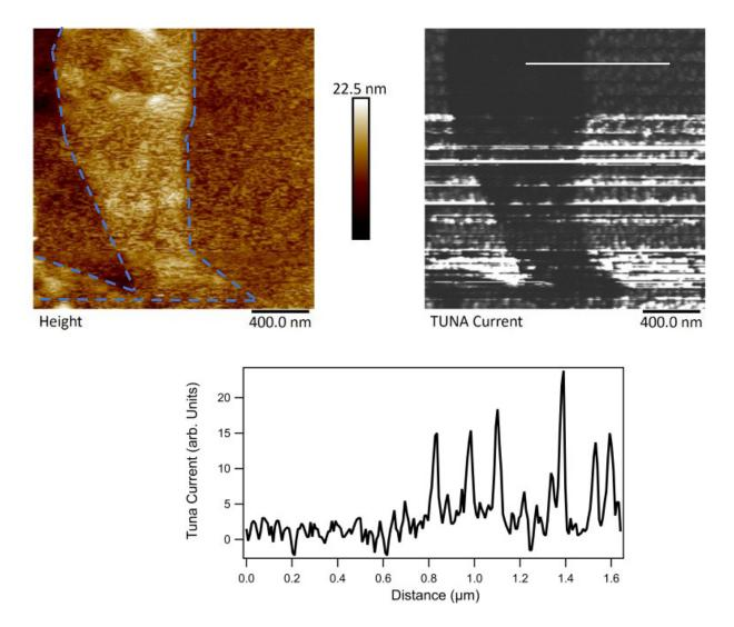
Figure S 21. APTES-rGO was deposited on Au coated Silicon. The flake is outlined by the blue dashed line. Peak force TUNA was used to map electrical conductivity of the flakes. As seen in the TUNA current map and section below, the APTES-rGO flake has limited conductivity which is increased in comparison to the GO flake which suggests some reduction has taken place in the APTES functionalisation process.
