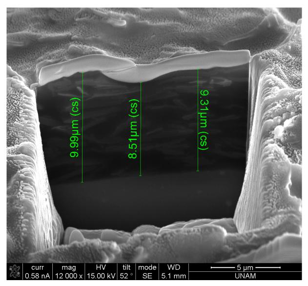
Figure S 32. SEM image of 10% APTES-rGO in coating.
