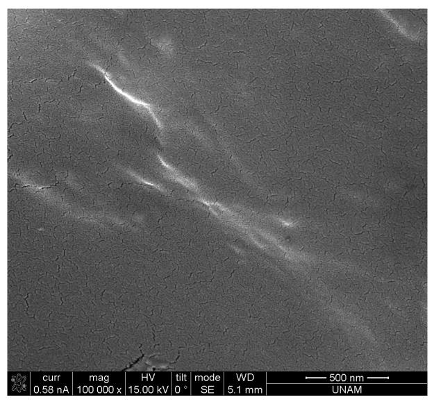
Figure S 27. SEM image of 10% APTES-rGO in coating.
