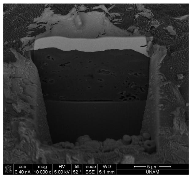
Figure S 41. SEM image of 5% rGO in coating.
