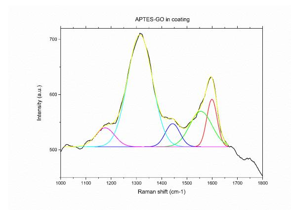
Figure S 9. Curve-fits to Raman spectra for APTES-rGO in coating. Gauss fits.
