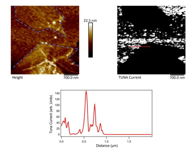
Figure S 20. GO was deposited on Au coated Silicon. The flake is outlined by the blue dashed line. Peak force TUNA was used to map electrical conductivity of the flakes using a PtIr tip. As seen in the TUNA current map. A section from the current map is also presented which shows no conductivity over the flake.
