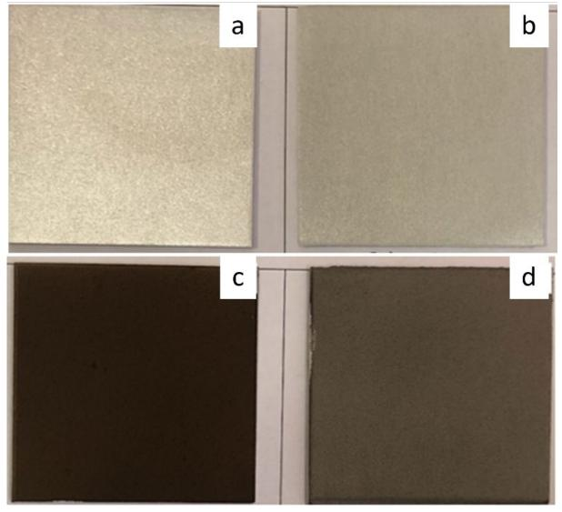
Figure S 19. Coatings on Al 2024 T-3. (a) no coating, (b) sol-gel only, (c) rGO in sol-gel, (d) APTES-rGO in sol-gel. Sample size 5×5 cm.
