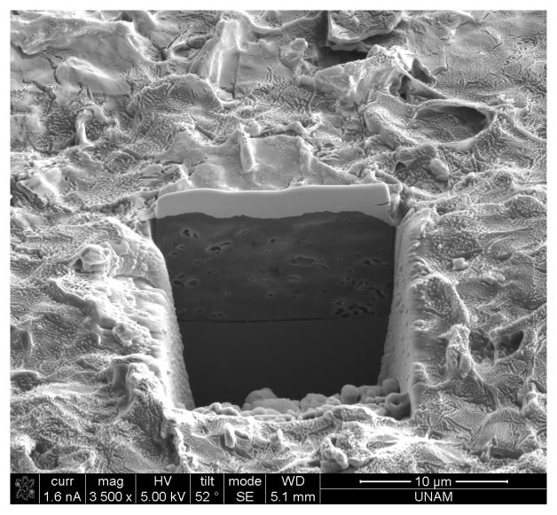
Figure S 36. SEM image of 5% rGO in coating.
