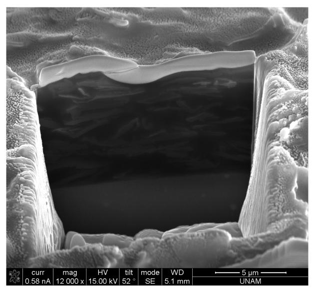
Figure S 31. SEM image of 10% APTES-rGO in coating.
