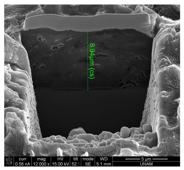
Figure S 39. SEM image of 5% rGO in coating.
