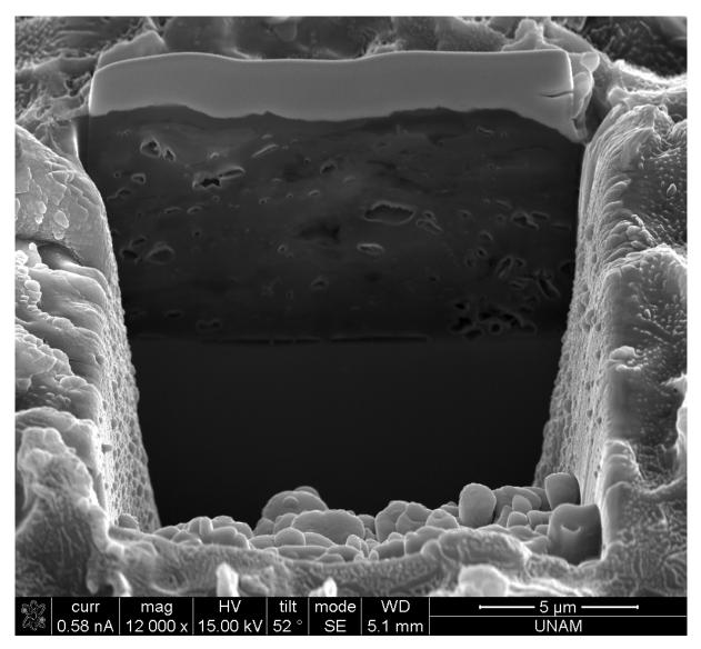
Figure S 38. SEM image of 5% rGO in coating.
