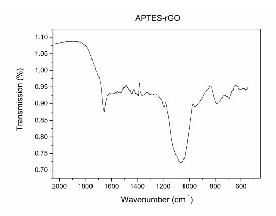
Figure S 3. FTIR spectrum of APTES-rGO.
