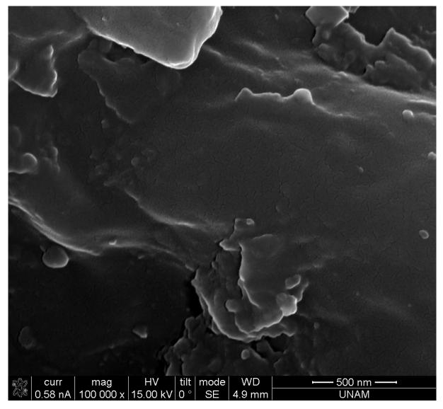
Figure S 35. SEM image of 5% rGO in coating.
