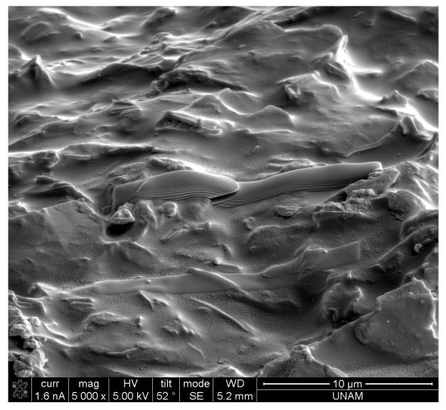
Figure S 26. SEM image of 10% APTES-rGO in coating.
