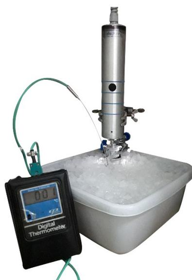
**Figure S1** Ice-cooled setup used for sonication of SWCNTs.
