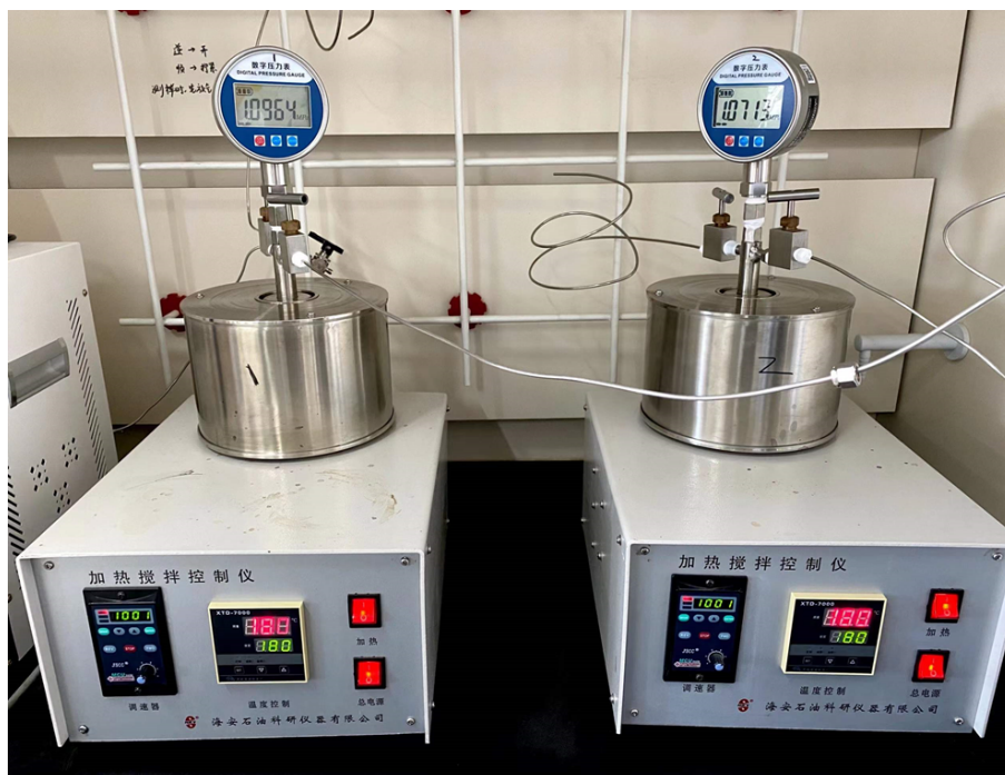
Figure S7. Experimental device for catalytic transfer hydrogenation of nitrobenzene.
