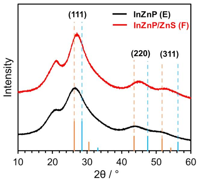
Supporting information figure 6: X-ray powder diffraction pattern and Miller indices of InZnP (E) and InZnP/ZnS (F) QDs. Bulk InP (orange trace) and bulk ZnS (blue trace) are shown for reference.
