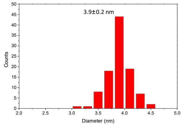
Supporting information figure 5: Particle size distribution of InZnP (C), (left hand side) and InZnP/ZnS (D) (right hand side) QDs.
