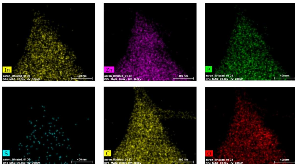
Supporting information figure 3: Elemental analysis of InZnP quantum dots (InZnP, grown at 45 minutes/120 °C followed by 10 minutes/220 °C) confirming the presence of elements consistent with the compound semiconductor, and a surface oxide species.
