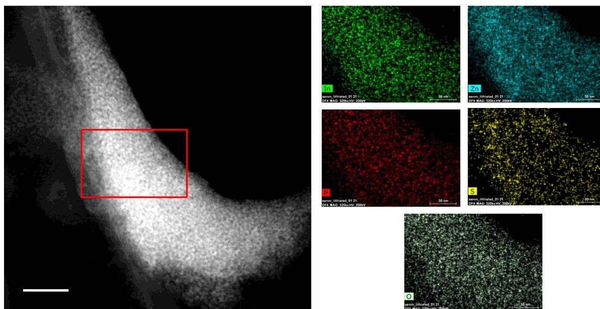
Supporting information figure 4: Electron microscopy and Elemental analysis for InZnP/ZnS particles (grown at 45 minutes/120 °C followed by 10 minutes/220 °C, followed by shell addition) scale bars = 30 nm.
