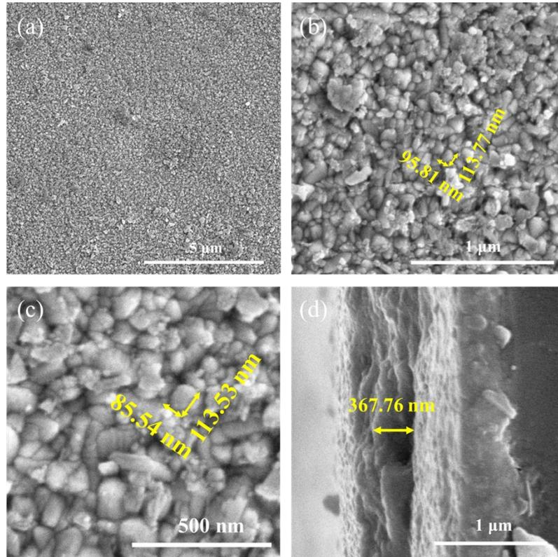
**Fig. S1** (a-c) Top SEM images and (d) sectional-view SEM image of NbSe<sub>2</sub>/Nb<sub>2</sub>O<sub>5</sub> metal-semiconductor heterostructure.
