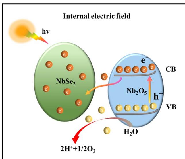
**Fig. S4** Schematic of charge transfer mechanism of NbSe<sub>2</sub>/Nb<sub>2</sub>O<sub>5</sub> under light irradiation
