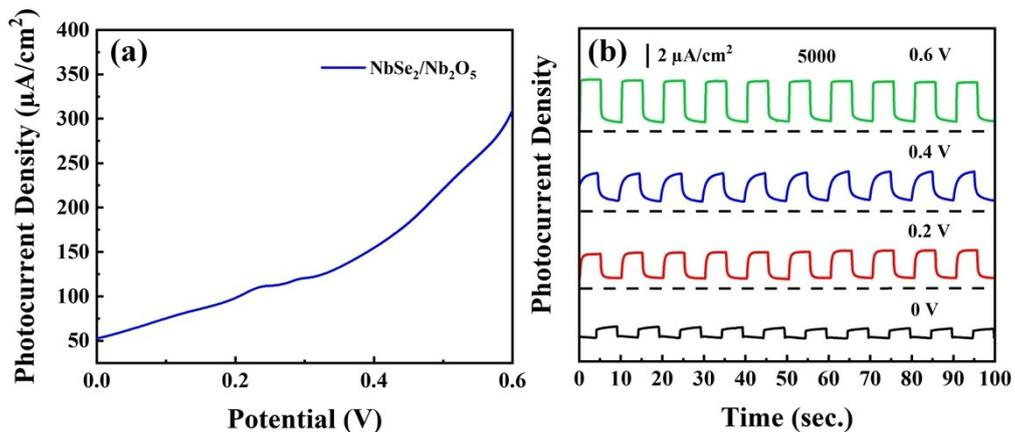
Fig. S3 (a) I-V curve from 0 to 0.6 V; (b) time-dependent photocurrent density under different applied voltage.
