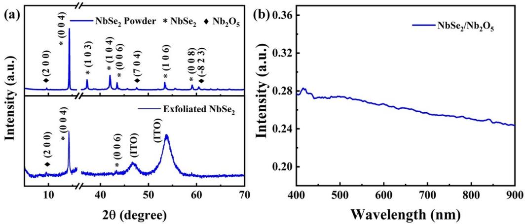
Fig. S2 (a) XRD pattern, and (b) UV-Vis absorption spectrum.
