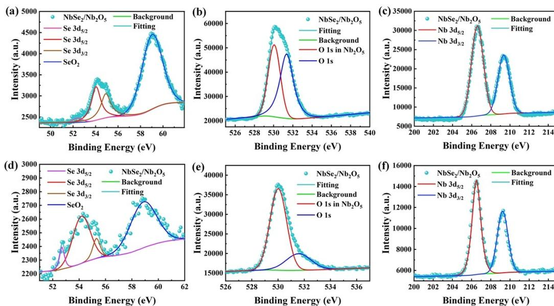
**Fig. S5** XPS signal of NbSe<sub>2</sub>/Nb<sub>2</sub>O<sub>5</sub> with (a) Se, (b) O, and (c) Nb elements after the measurement; XPS signal of NbSe<sub>2</sub>/Nb<sub>2</sub>O<sub>5</sub> nanosheets with (d) Se, (e) O, and (f) Nb elements in enough oxygen condition.
