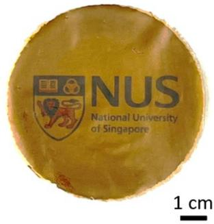
**Supplementary Figure 3.** A transparent and robust large-scale GGC<sub>5</sub> membrane, diameter: 8 cm.
