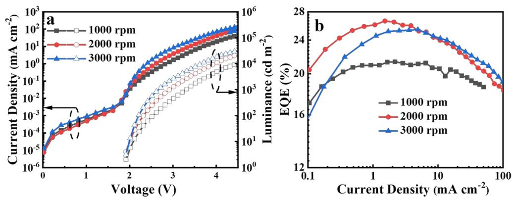
Figure S2. (a)  $J$ - $V$ - $L$  and (b) EQE curves of the PEABr-based devices with different spin-coating speed of the PEABr layer.
