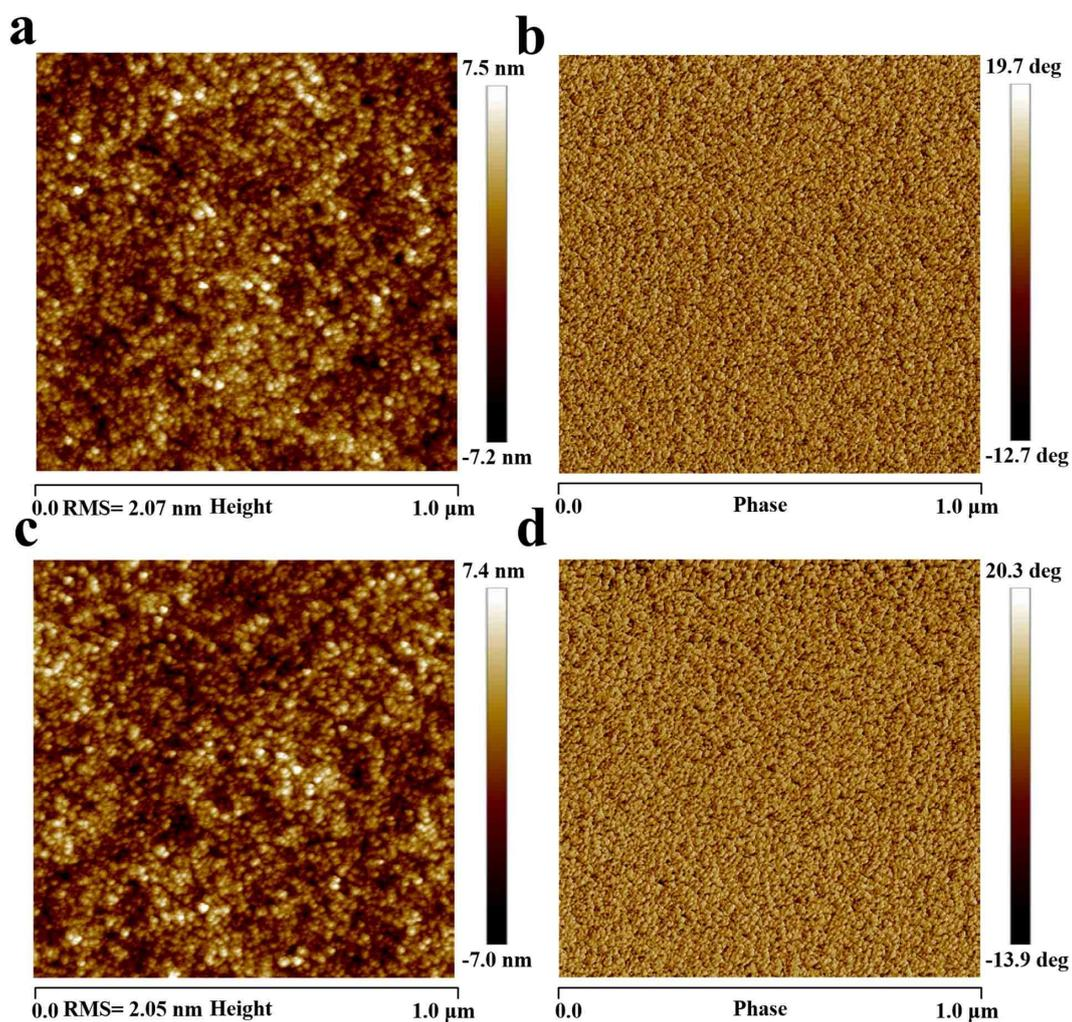
Figure S1. AFM images of ZnMgO film captured in contact (a) and phase mode (b), respectively. AFM images of PEABr/ZnMgO film captured in contact (c) and phase mode (d), respectively.
