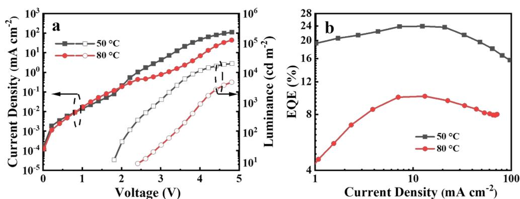
Figure S3. (a)  $J$ - $V$ - $L$  and (d) EQE curves of the devices with PEABr annealed at 50 °C and 80 °C, respectively.
