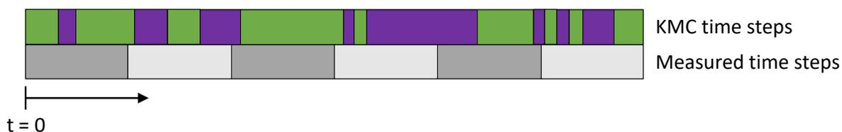
**Fig. S10:** Equidistant measurement time steps of the source-measure-unit compared with the event-driven time steps of the KMC simulation. Each KMC time step contains one vacancy diffusion instance with a respective current amplitude change. The measured time steps superimpose the current change of several vacancy diffusion instances occurring in the given time frame.
