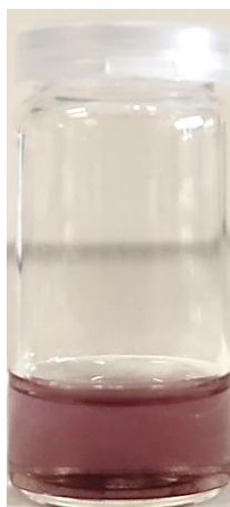
Figure S12. Representative photograph of the resulting TIPS-GNR (10) dispersion in THF after sonication.
