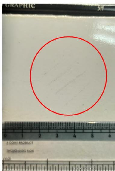
**Fig. S8** Evaluation of hardness of RT coated tiles surface using pencil hardness tester (BYK Gardner instrument).
