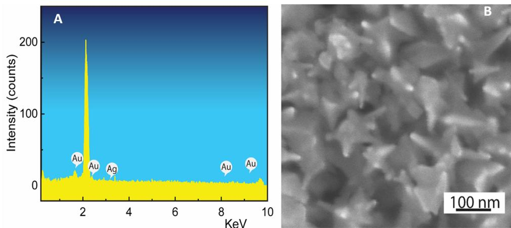
**Fig. S2 (A)** Energy dispersive X-Ray spectroscopy (EDS) and **(B)** scanning electron microscopy (SEM) of formed SG NPs.
