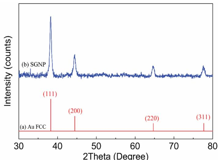
**Fig. S3** X-Ray diffraction pattern of (a) Au fcc crystal and (b) as-synthesized SGNPs.
