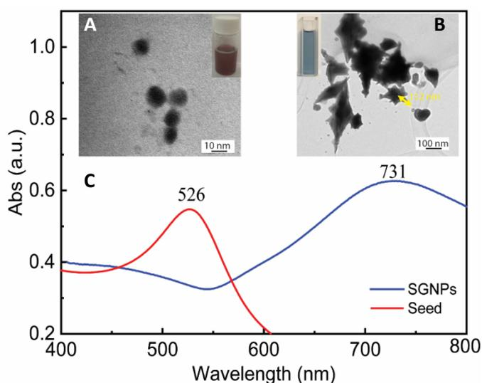
**Fig. S1** The TEM images of (A) seed nanoparticles with the corresponding SGNPs colloidal solution (right inset) (scale bar 10 nm), (B) the formed SGNPs with corresponding blue colloid (left inset) (scale bar 100 nm), (C) UV-Vis spectroscopy of seed and SGNPs colloidal solutions
