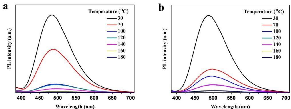
Fig. S31 The PL spectra of (a) 381F and (b) 381H PDMS film excited at 365 nm.
