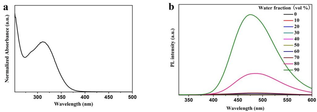
Fig. S3 (a) Absorption spectrum of **381F** in THF solution and (b) PL intensity spectra of **381F** in tetrahydrofuran/water mixtures with different water fractions.
