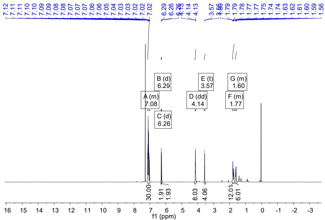
$^1\text{H}$ -NMR spectrum of compound **361H** ( $\text{CDCl}_3$ , 600MHz)
