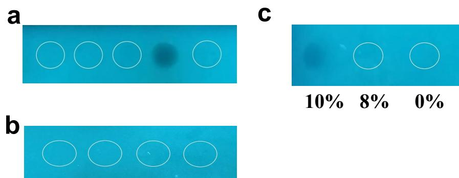
Fig. S26 The film of **341F** with solvent from left to right: a) benzene, toluene, phenylcarbinol, benzaldehyde, benzoic acid (these compounds are dissolved in ethyl acetate in 2 mg/mL), b) acetonitrile, acetic acid, ethanol, ethyl acetate, c) benzaldehyde fraction in benzene/ethyl acetate (v/v).
