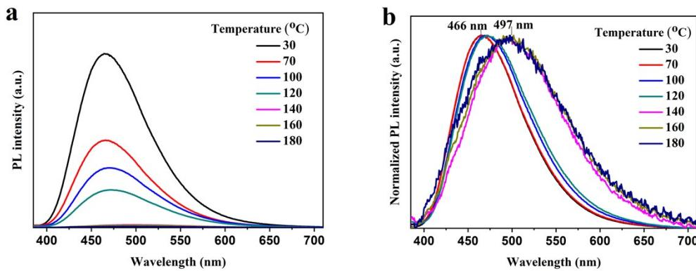
Fig. S32 (a) The PL spectra and (b) normalized PL spectra of pure original 361F solid excited at 365 nm.
