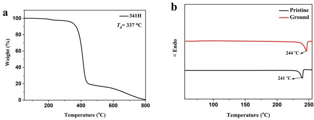
Fig. S19 (a) TGA and (b) DSC curves of 341H.
