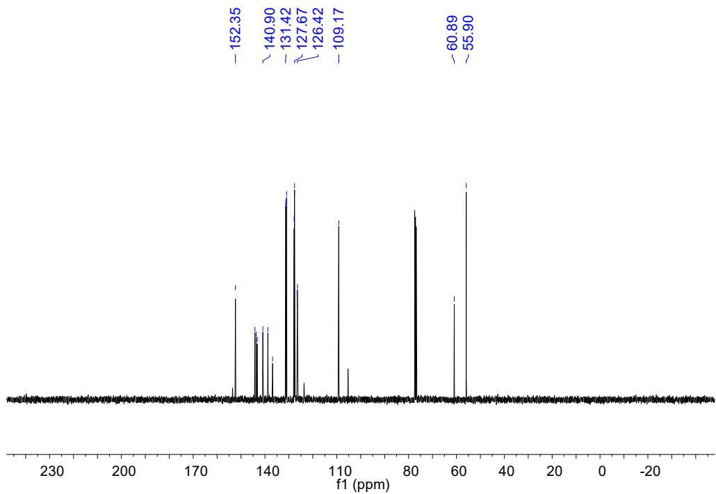
$^{13}\text{C}$ -NMR spectrum of compound **1** ( $\text{CDCl}_3$ , 600MHz)
