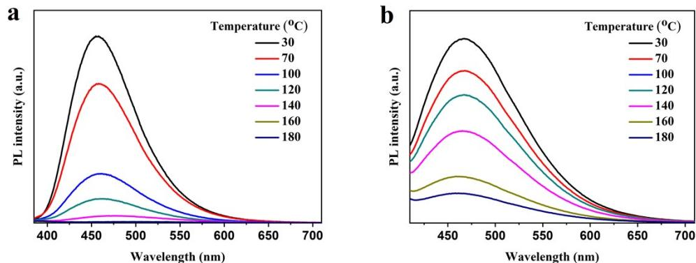
Fig. S30 The PL spectra of (a) 361F and (b) 361H PDMS film excited at 365 nm.
