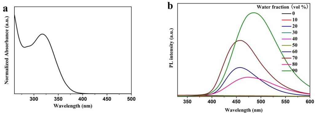
Fig. S8 (a) Absorption spectrum of **362H** in THF solution and (b) PL intensity spectra of **362H** in tetrahydrofuran/water mixtures with different water fractions.
