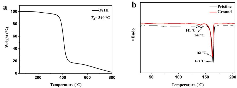
Fig. S21 (a) TGA and (b) DSC curves of 381H.
