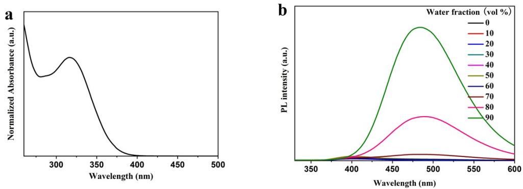
Fig. S7 (a) Absorption spectrum of **342H** in THF solution and (b) PL intensity spectra of **342H** in tetrahydrofuran/water mixtures with different water fractions.
