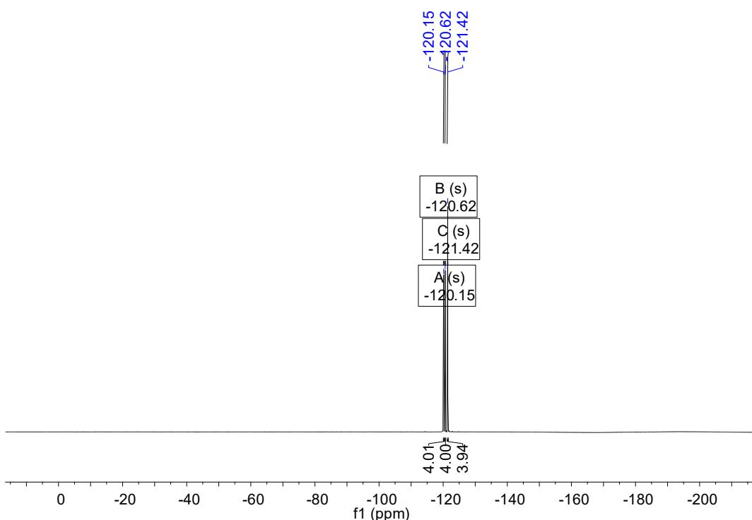
$^{19}\text{F}$ -NMR spectrum of compound **341F** ( $\text{CDCl}_3$ , 600MHz)
