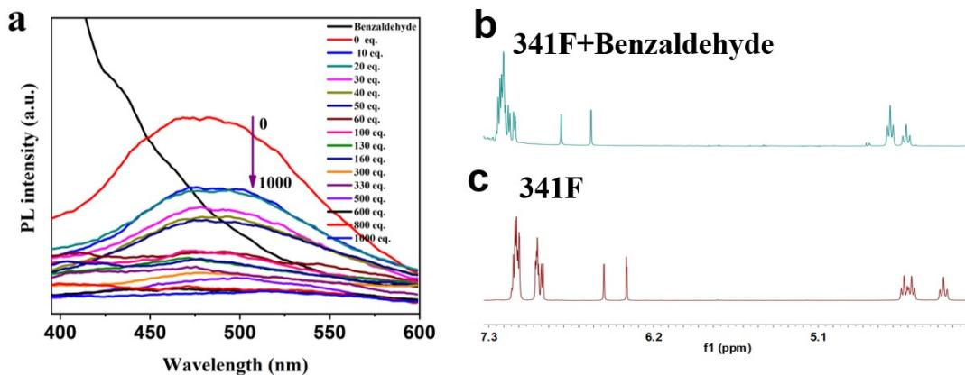
Fig. S27 (a) PL intensity spectra of the **341F** solution ( $1 \times 10^{-4}$  M) upon adding molar equivalent of benzaldehyde from 10 to 1000, the partial <sup>1</sup>H NMR spectra of (b) a mixture of **341F** and benzaldehyde (mol ratio, **341F** : benzaldehyde = 1 : 100) and (c) pure **341F** (DMSO-d<sub>6</sub>, 600 MHz).
