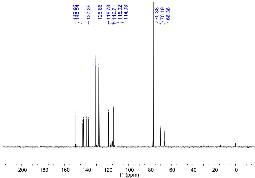
$^{13}\text{C}$ -NMR spectrum of compound **341F** ( $\text{CDCl}_3$ , 600MHz)
