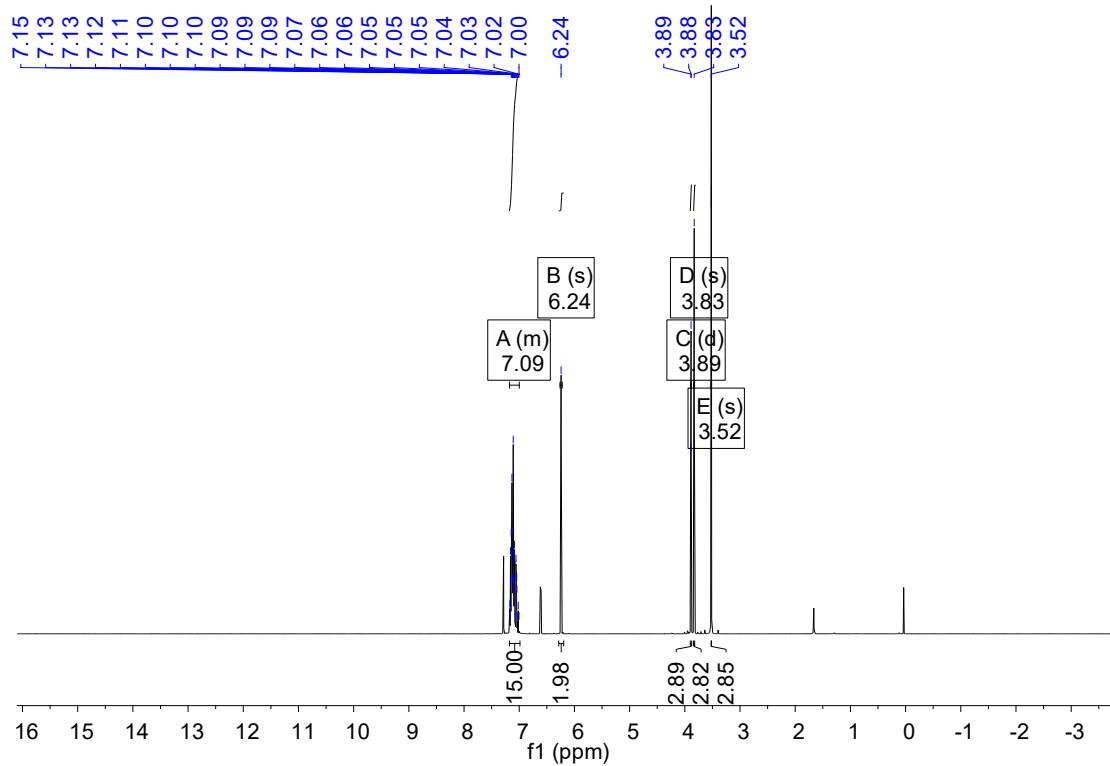
$^1\text{H}$ -NMR spectrum of compound **1** ( $\text{CDCl}_3$ , 600MHz)
