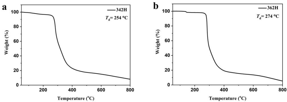
Fig. S22 TGA curves of (a) 342H and (b) 362H, respectively.
