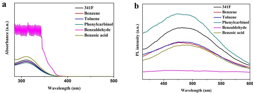
Fig. S25 (a) Absorption spectrum and (b) PL intensity spectra of benzene derivates in **341F** solution ( $1 \times 10^{-4}$  M, benzene derivates: **341F** solution = 1:100 (v/v)).
