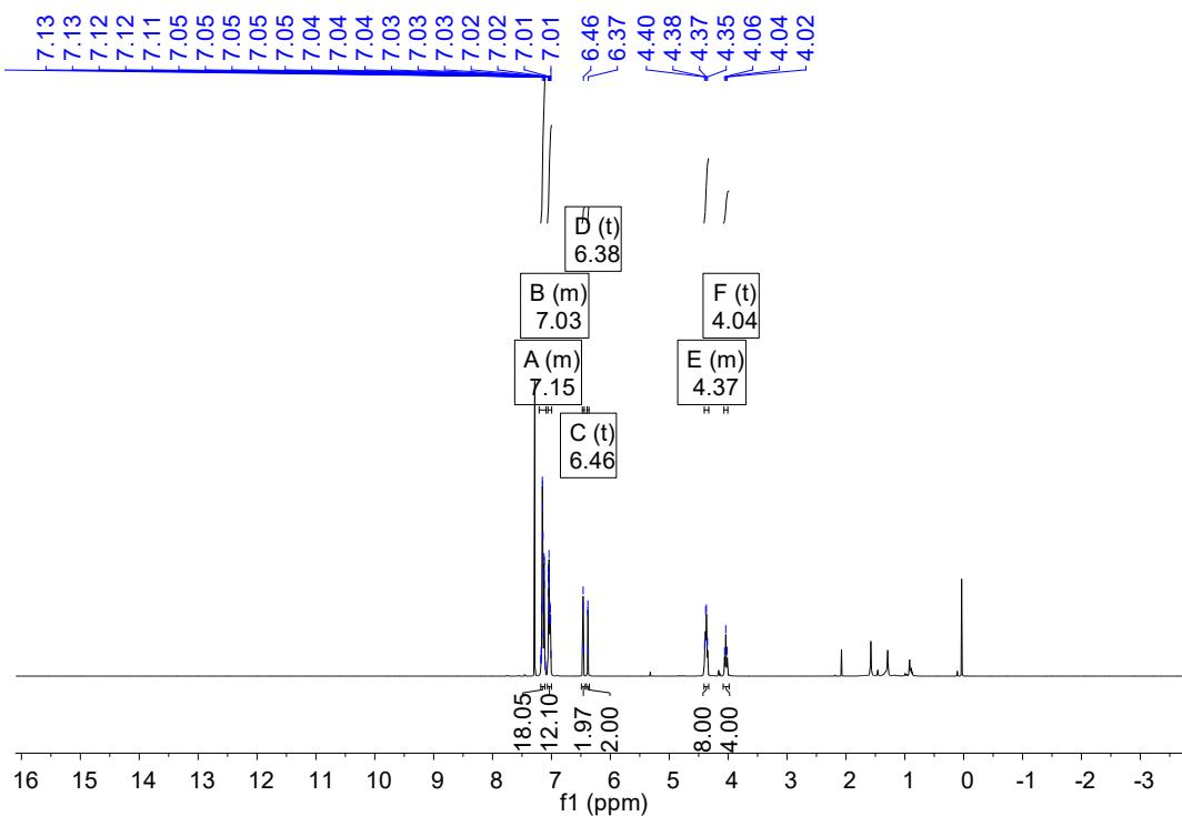
$^1\text{H}$ -NMR spectrum of compound **341F** ( $\text{CDCl}_3$ , 600MHz)
