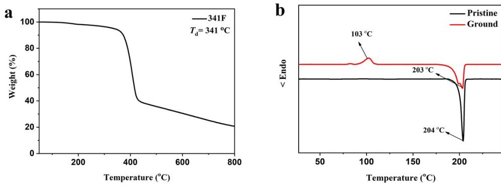
Fig. S16 (a) TGA and (b) DSC curves of **341F**.
