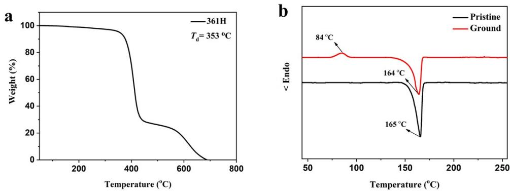
Fig. S20 (a) TGA and (b) DSC curves of 361H.
