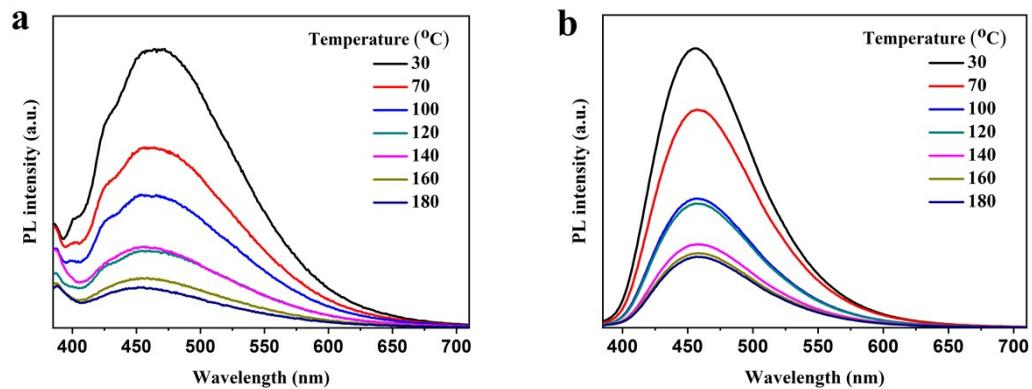
Fig. S29 The PL spectra of (a) 341F and (b) 341H PDMS film excited at 365 nm.
