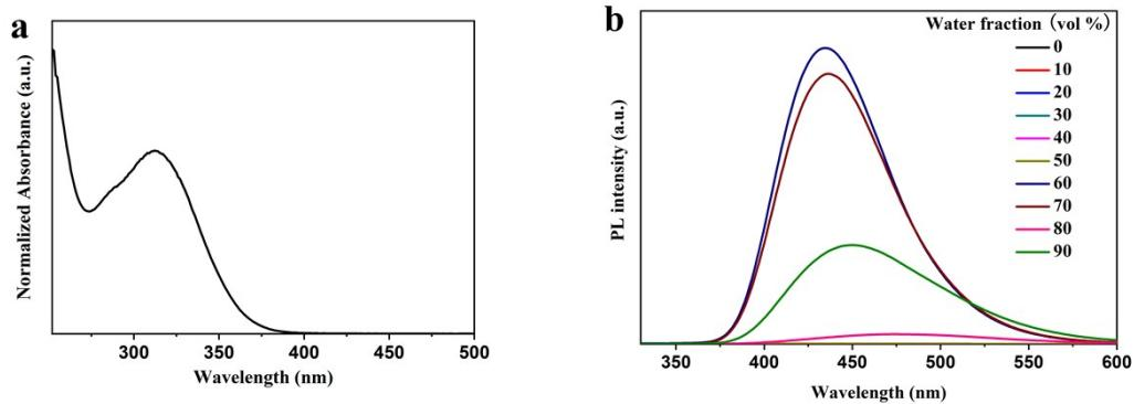
Fig. S1 (a) Absorption spectrum of **341F** in THF solution and (b) PL intensity spectra of **341F** in tetrahydrofuran/water mixtures with different water fractions.
