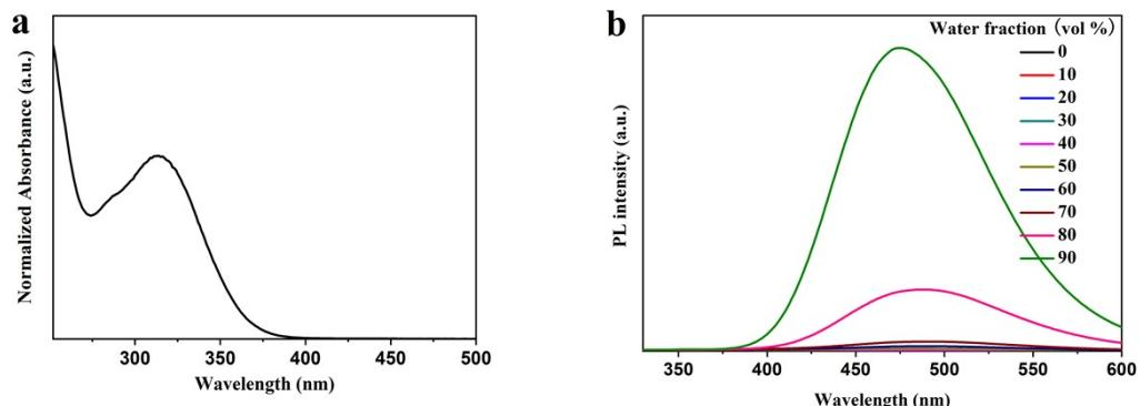
Fig. S2 (a) Absorption spectrum of **361F** in THF solution and (b) PL intensity spectra of **361F** in tetrahydrofuran/water mixtures with different water fractions.
