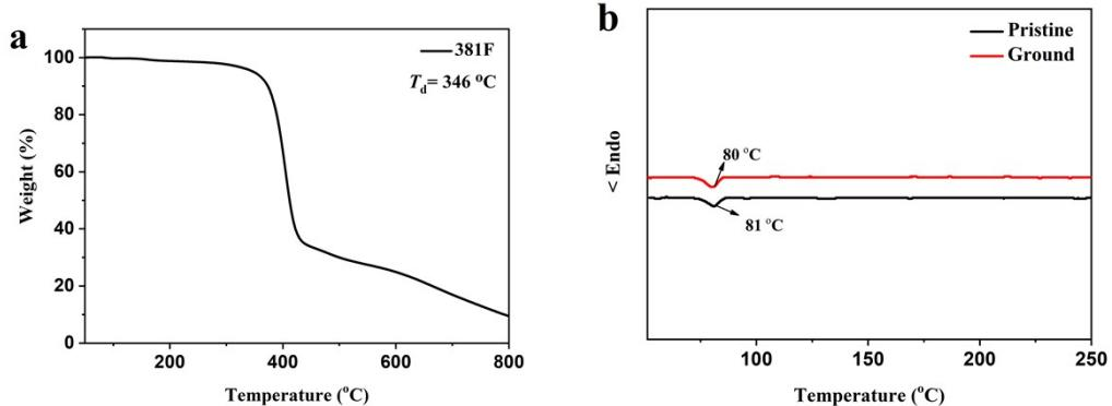
Fig. S18 (a) TGA and (b) DSC curves of **381F**.
