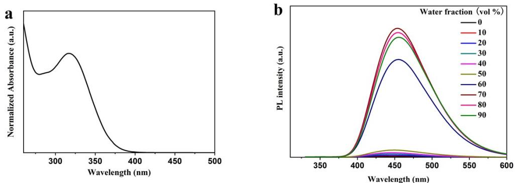
Fig. S4 (a) Absorption spectrum of **341H** in THF solution and (b) PL intensity spectra of **341H** in tetrahydrofuran/water mixtures with different water fractions.
