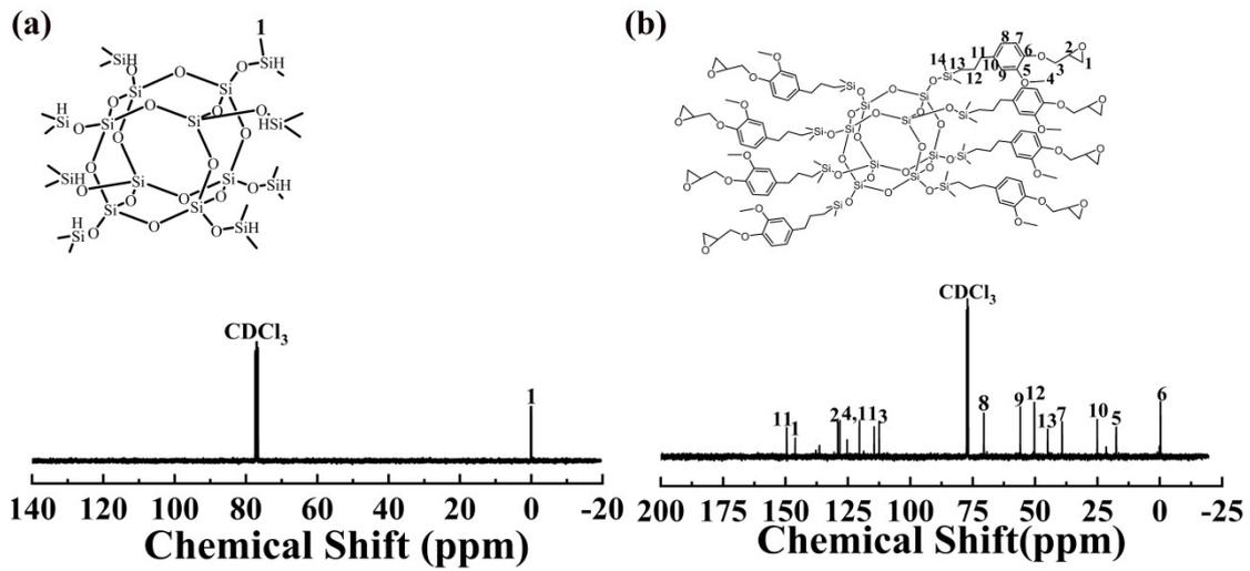
**Fig. S4.** <sup>13</sup>C-NMR spectra of (a) POSS-H and (b) SHEP samples.
