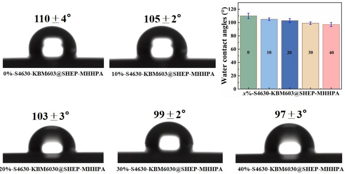
**Fig. S9.** Water contact angle images of  $x\%$ -S4630-KBM603@SHEP-MHHPA.
