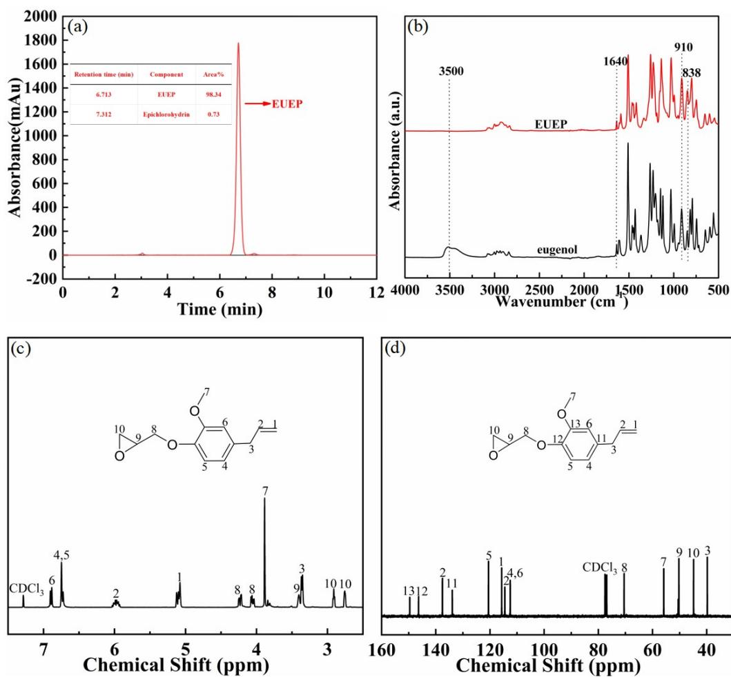
**Fig. S3.** (a) HPLC spectrum of product after epoxidation reaction of eugenol; (b) FTIR spectra of eugenol and EUEP; (c) <sup>1</sup>H-NMR and (d) <sup>13</sup>C-NMR spectra of EUEP.
