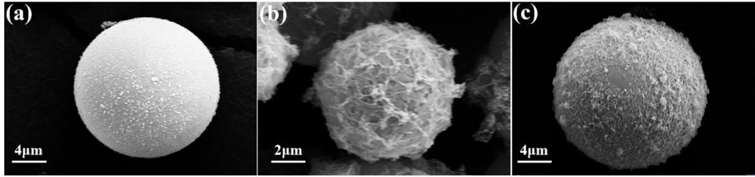
**Fig. S5.** SEM images of the (a) original S4630, modified S4630: (b) non-ultrasonic treatment and (c) ultrasonic treatment.
