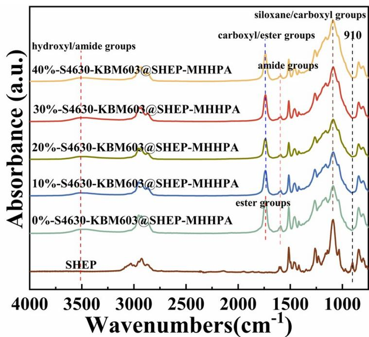
**Fig. S7.** FTIR spectra (epoxy before and after curing).
