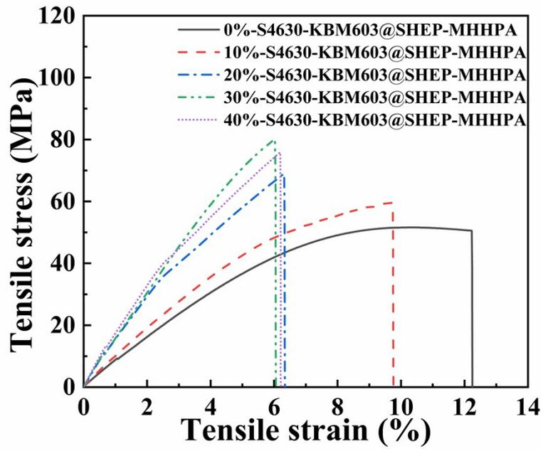
**Fig. S6.** Stress-strain curves of  $x\%$ -S4630-KBM603@SHEP-MHHPA.
