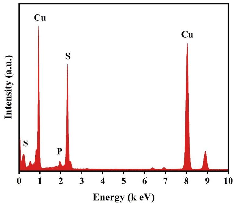
**Fig. S3** Energy dispersive X-ray (EDX) spectrum of 0.03P-CuS.
