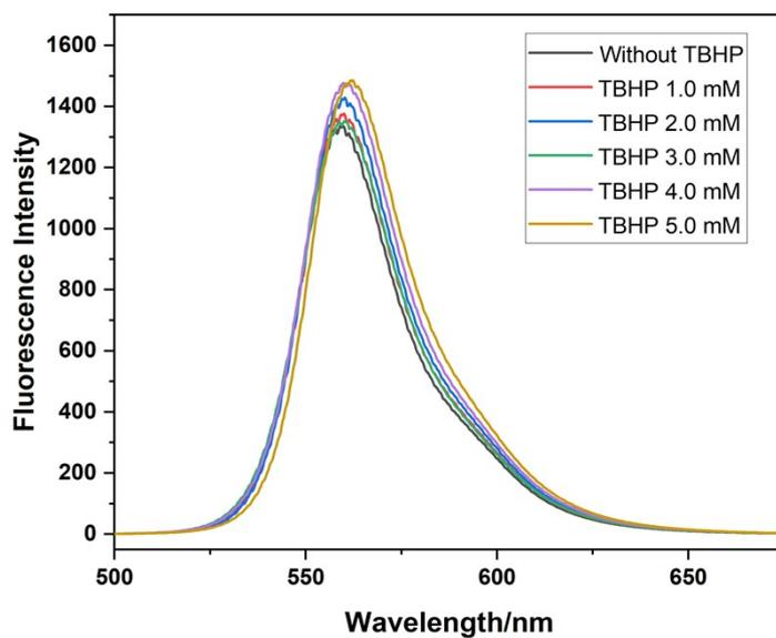
**Figure S9** Fluorescence emission spectra of Na<sub>2</sub>-eosin Y ( $5 \times 10^{-4}$  M) in THF with TBHP (1.0 - 5.0 mM)
