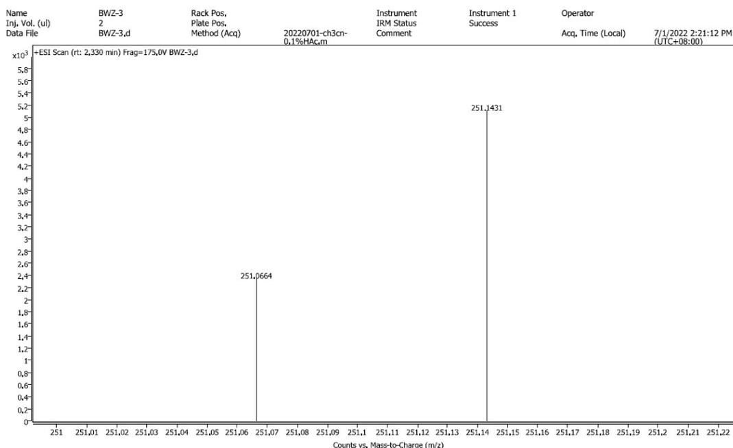
**Figure S7** HRMS spectrum of the  $\alpha$ -alkoxyalkyl radical / ASYM adduct **10**
