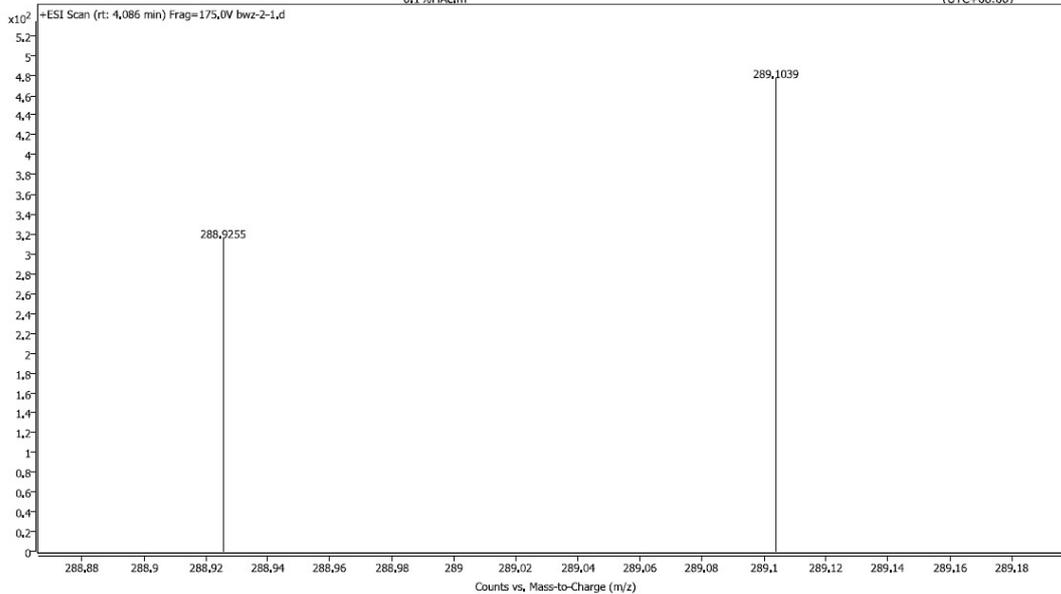
**Figure S5** HRMS Spectrum of the benzenesulfenyl radical /ASYM adduct **8**
