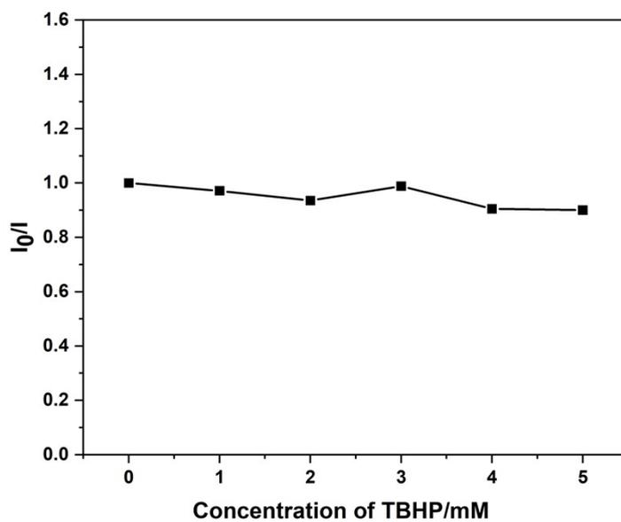
**Figure S10** The linear relationship between  $I_0/I$  ( $I_0$  and  $I$  are the fluorescence intensities before and after the addition of TBHP) and the concentration of TBHP
