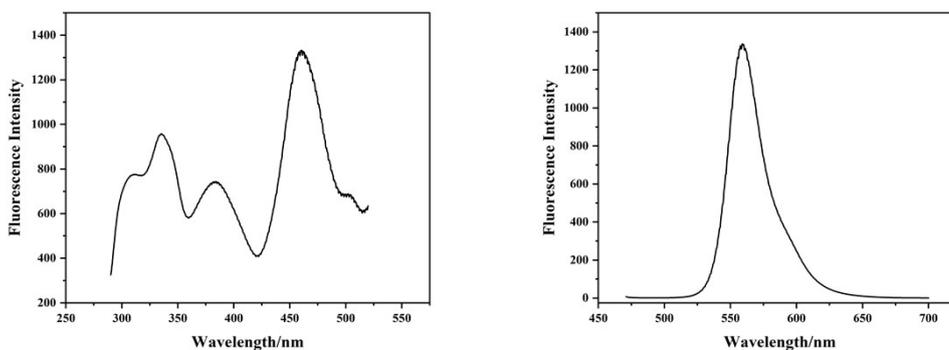
**Figure S8** Fluorescence excitation (left) and emission (right) spectra of Na<sub>2</sub>-eosin Y ( $5 \times 10^{-4}$  M) in THF
