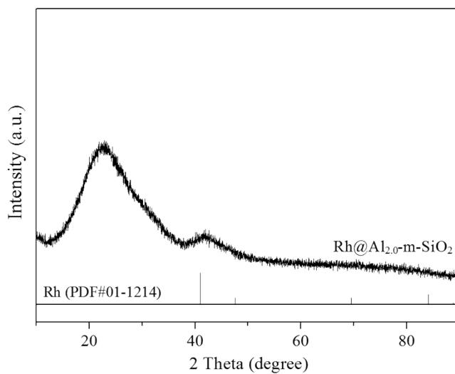
**Figure S9.** XRD pattern of Rh@Al<sub>0.25</sub>-mSiO<sub>2</sub> after five cycle experiments.
