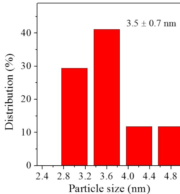
**Figure S8.** Size distribution of Rh@Al<sub>2.0</sub>-mSiO<sub>2</sub> after five recycling experiments.
