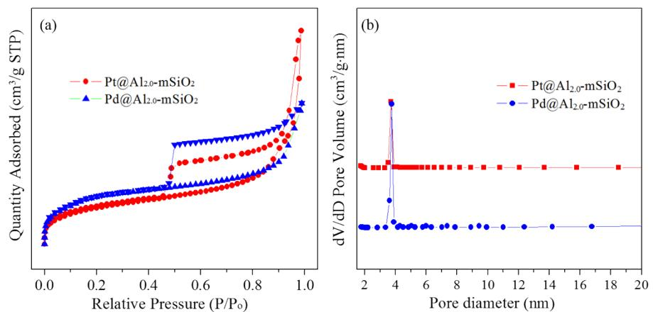
**Figure S6.** a) N<sub>2</sub> adsorption-desorption isotherms of Pt@Al<sub>2.0</sub>-mSiO<sub>2</sub> and Pd@Al<sub>2.0</sub>-mSiO<sub>2</sub> and b) their corresponding pore size distributions.
