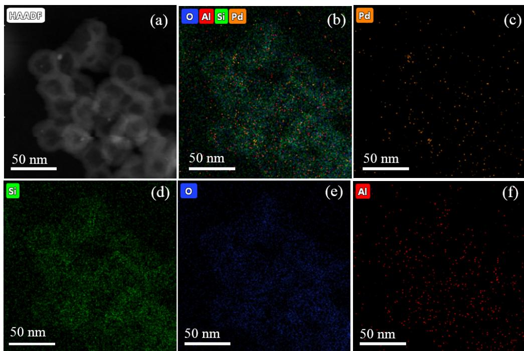
**Figure S4.** HAADF-STEM images of Pd@Al-mSiO<sub>2</sub> samples: (a) area selected for phase mapping; (b) combined phase mapping of Pd, Si, O and Al; (c) Pd phase mapping; (d) Si phase mapping; (e) O phase mapping; and (f) Al phase mapping.
