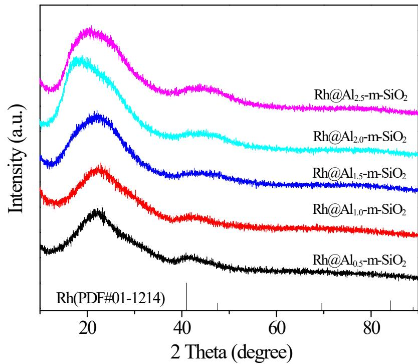
**Figure S2.** XRD patterns of Rh@Al<sub>0.5</sub>-m-SiO<sub>2</sub>, Rh@Al<sub>1.0</sub>-m-SiO<sub>2</sub>, Rh@Al<sub>1.5</sub>-m-SiO<sub>2</sub>, Rh@Al<sub>2.0</sub>-m-SiO<sub>2</sub>, and Rh@Al<sub>2.5</sub>-m-SiO<sub>2</sub>.
