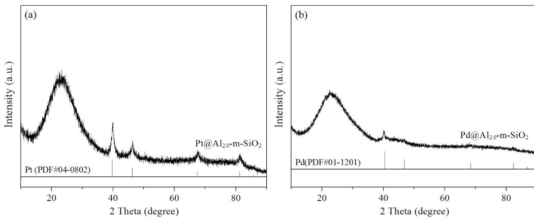
**Figure S3.** XRD profiles of Pt@Al<sub>2</sub>-mSiO<sub>2</sub> and Pd@Al-mSiO<sub>2</sub> samples.
