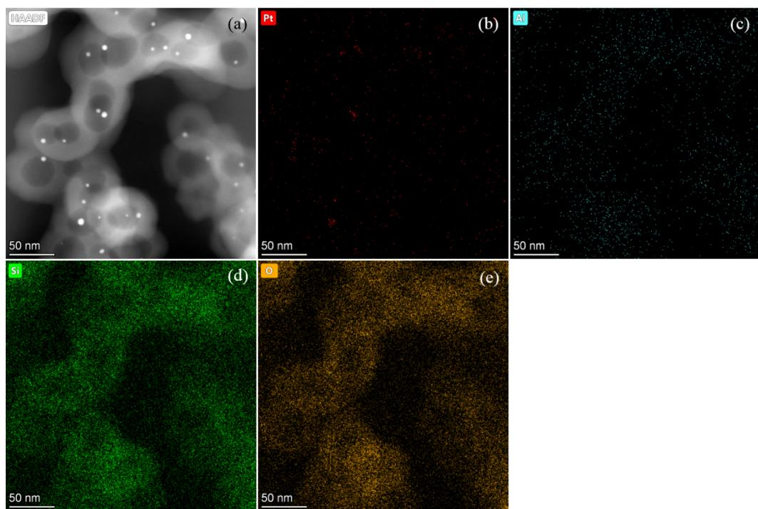
**Figure S5.** HAADF-STEM images of Pd@Al-mSiO<sub>2</sub> samples: (a) area selected for phase mapping; (b) Pt phase mapping; (c) Al phase mapping; (d) Si phase mapping; and (e) O phase mapping.
