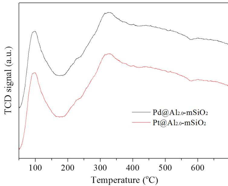
**Figure S7.** NH<sub>3</sub>-TPD profiles of Pd@Al<sub>2.0</sub>-mSiO<sub>2</sub> and Pt@Al<sub>2.0</sub>-mSiO<sub>2</sub> catalysts.
