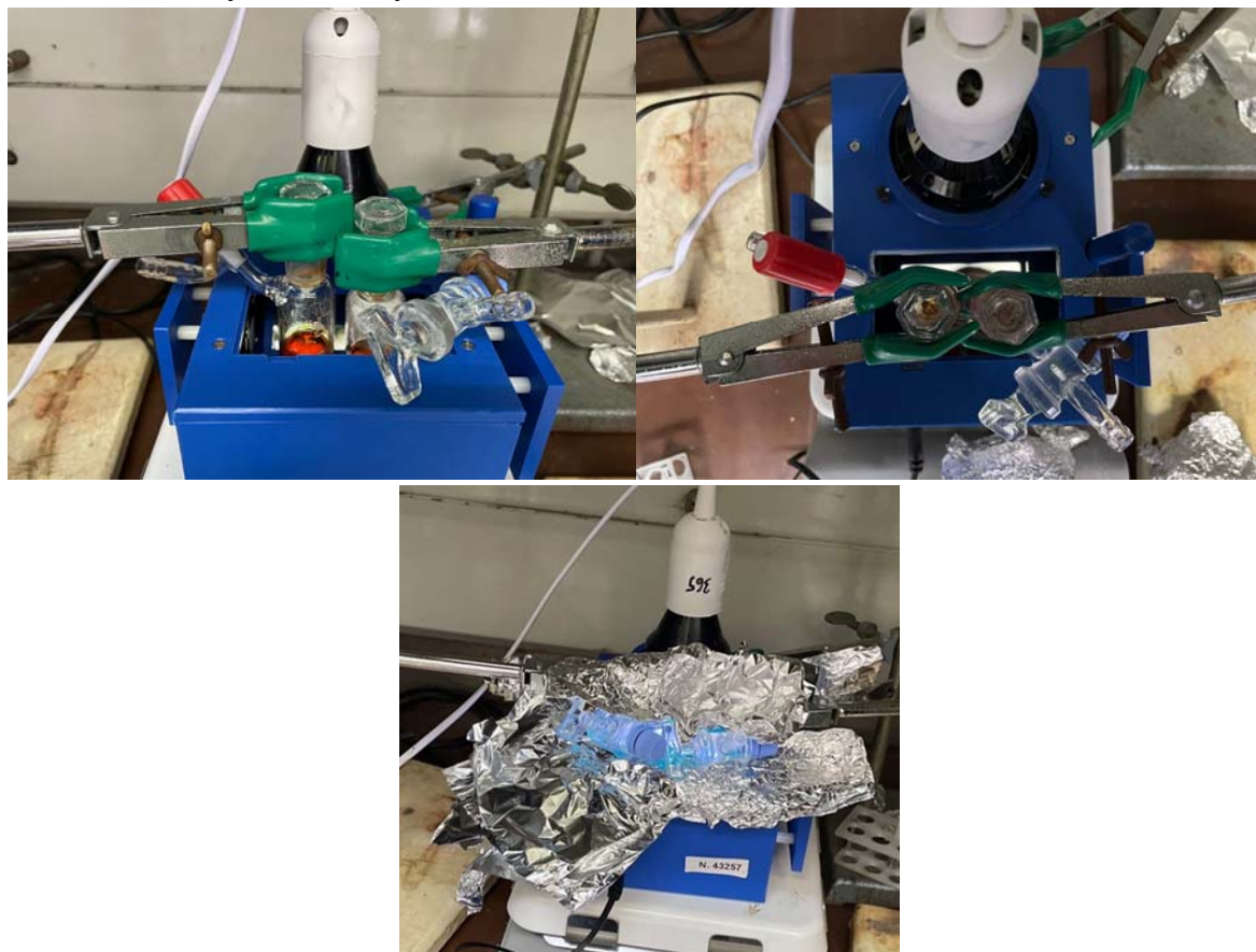
Figure S6. Photochemical set-up. Examples of large-scale reactions. Reaction. Up - solutions of compounds 5a and 4 with 405 nm LED lamp before irradiation. Down - solutions of compounds 1e and 1f with 365 nm LED lamp upon irradiation.
