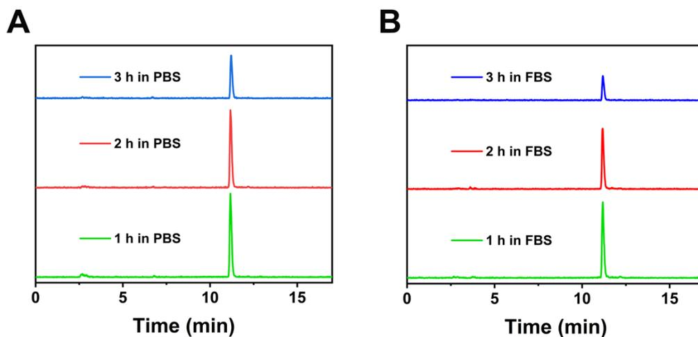
**Fig. S10.** Stability experiment of  $[^{68}\text{Ga}]\text{Nap-1G}$  in PBS (A) and FBS (B) after incubating 1, 2, 3 h, monitoring by a radio-HPLC.
