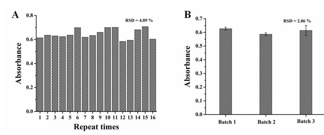
**Figure S12.** (A) The reproducibility testing and (B) the batch-to-batch repeatability of the Fe NPs nanozyme for colorimetric detection of xanthine (50  $\mu$ M).
