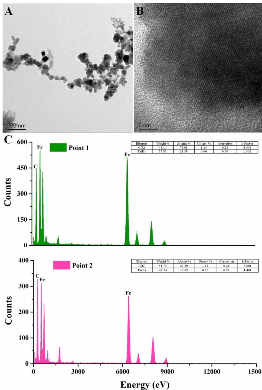
**Figure S1.** (a) TEM and (b) HRTEM images of Fe NPs. (c) EDX spectra of different points of outer shell of Fe NPs.
