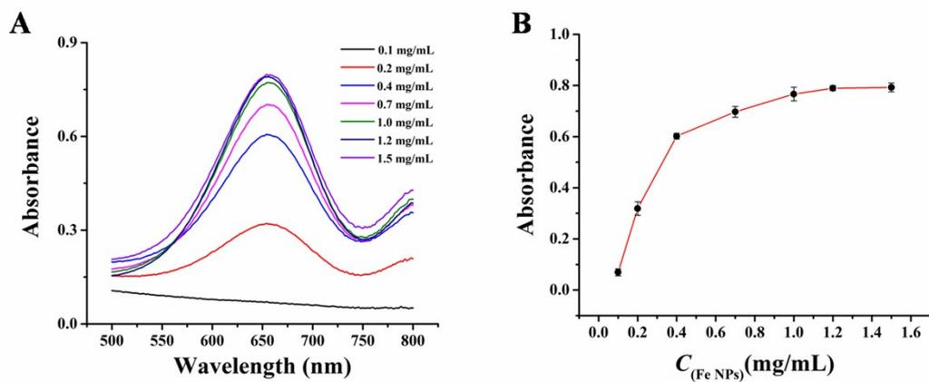
**Figure S9.** UV-vis absorption spectra of (A) concentration of Fe NPs nanozyme. Optimum conditions for xanthine response based on the Fe NPs nanozyme sensing platform. (B) concentration of Fe NPs nanozyme. The error bar represents the deviation of three determinations.
