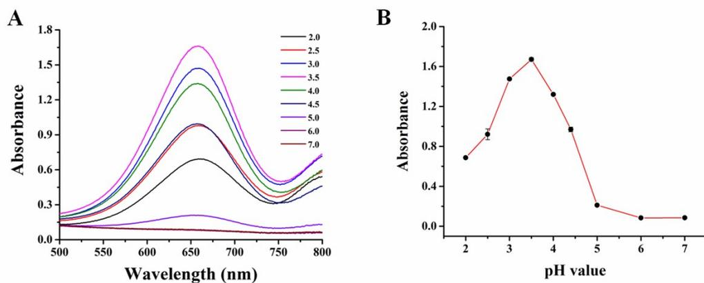
**Figure S6.** UV-vis absorption spectra of (A) pH value of Fe NPs nanoenzyme. Optimum conditions for xanthine response based on the Fe NPs nanozyme sensing platform. (B) pH value of the Fe NPs nanozyme. The error bar represents the deviation of three determinations.
