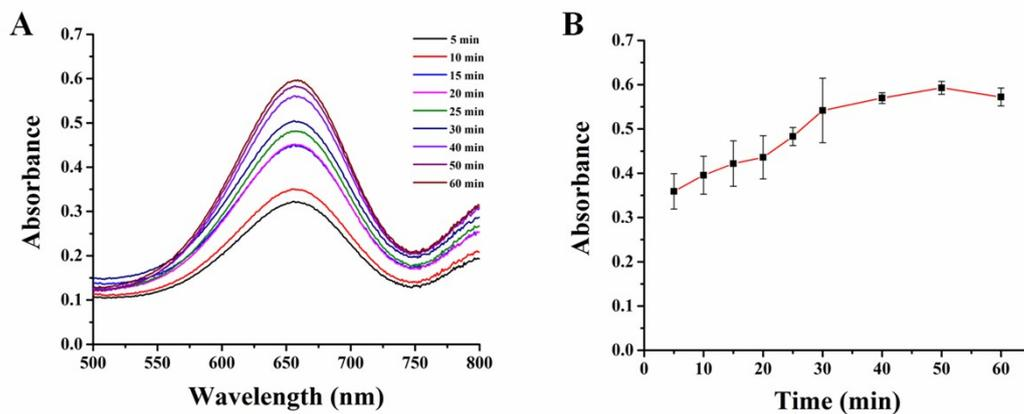
**Figure S8.** UV-vis absorption spectra of (A) incubation time between XOD and xanthine. Optimum conditions for xanthine response based on the Fe NPs nanozyme sensing platform. (B) incubation time between XOD and xanthine. The error bar represents the deviation of three determinations.
