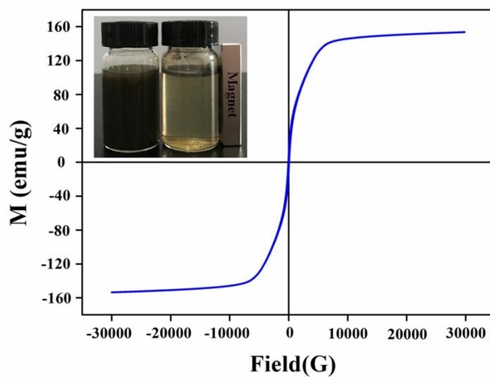
**Figure S2.** Magnetic hysteresis curve of Fe NPs. Inset: pictures of Fe NPs in solution with and without a magnet.
