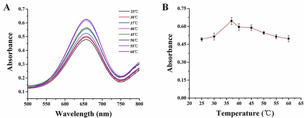
**Figure S7.** UV-vis absorption spectra of (A) incubation temperature between XOD and xanthine. Optimum conditions for xanthine response based on the Fe NPs nanozyme sensing platform. (B) incubation temperature between XOD and xanthine. The error bar represents the deviation of three determinations.
