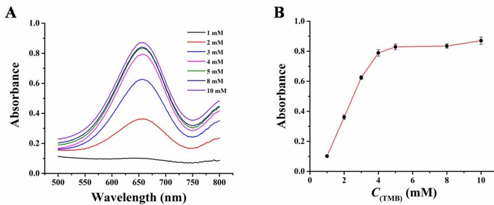
**Figure S10.** UV-vis absorption spectra of (A) concentration of TMB. Optimum conditions for xanthine response based on the Fe NPs nanozyme sensing platform. (B) concentration of TMB. The error bar represents the deviation of three determinations.
