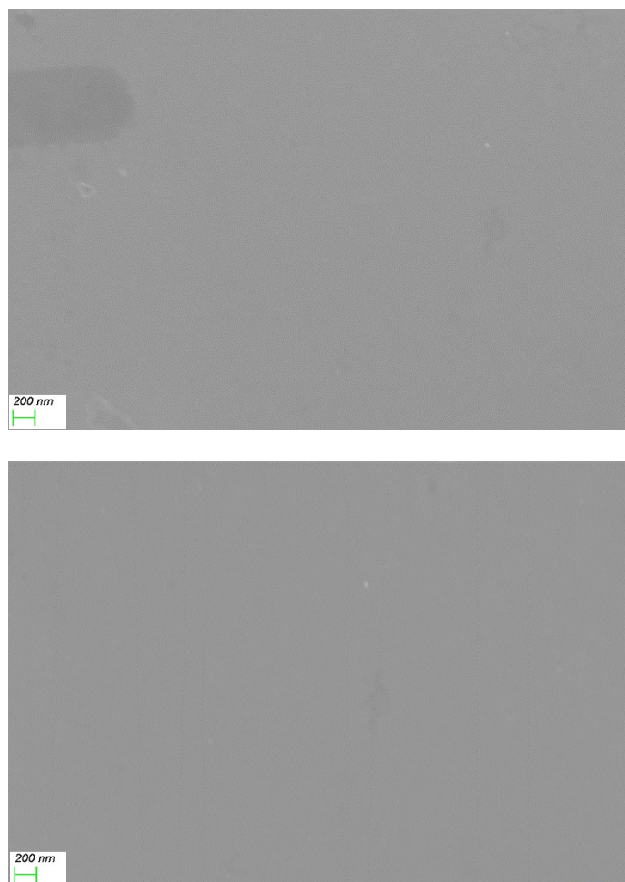
Fig. S14 SEM images of the surface of ITO electrode before (top) and after (bottom) 4 h CPE experiments (1.42 V vs. NHE) of 0.2 mM of 1 in 0.1 M PBS at pH 8.0.
