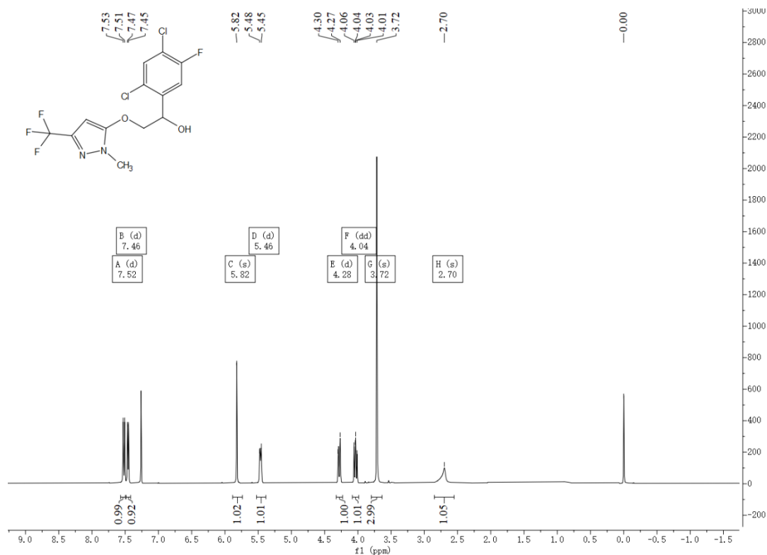
Figure 46. 1 H NMR spectrum of target compound 6p
